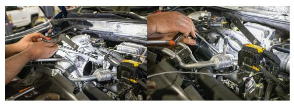
6. Remove factory intake horn.
