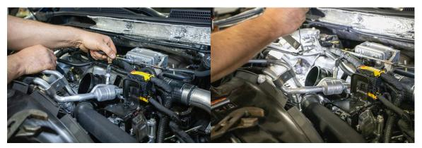
5. Remove two 13 mm head bolts holding the turbo inlet horn to turbo using a long extension and swivel socket (1/4" drive).
