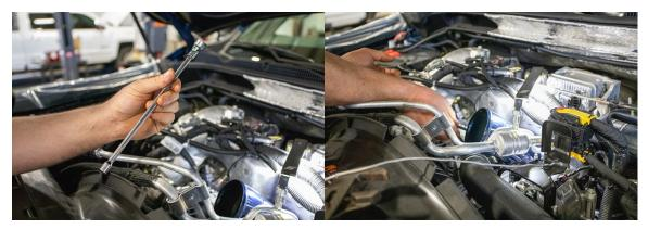
11. Reinstall the air box, intake tube and any other parts removed for the install.
