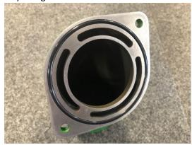
8. Install O-ring into the groove of your new intake horn using a very small amount of grease to hold in place if needed on the pipe and seals to prevent damage / nicks during installation.
