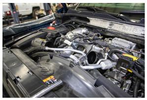
3. Unplug MAF sensor and remove 8 mm screws holding the lid onto the airbox.
