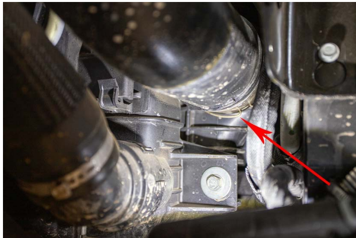
29. Using a pick or flat blade screwdriver, remove clip at lower intercooler pipe connection and pop pipe off of intercooler.
