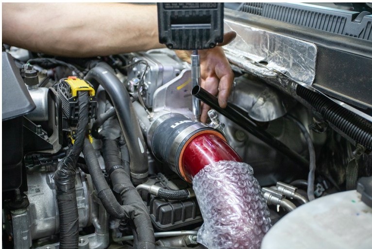
13. Check for proper engagement of pipe at both boots and tighten all clamps making sure that the clamps are placed just behind the pipe bead roll and square to prevent boost leaks.
