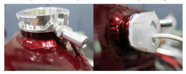
12. Install new tank. Use lower existing stud & new 6mm bolt in threaded hole in fender.
