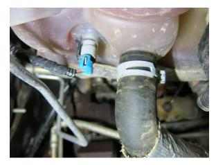
9. Remove the coolant tank nuts.
