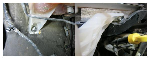
10. Remove the coolant tank.
