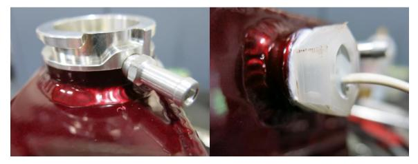
12. Install new tank. Use lower existing stud & new 6mm bolt in threaded hole in fender.
