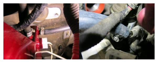
16. Install the overflow hose and route it down into the fender area.
