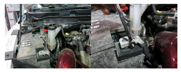
2. Drain coolant. This is at the driver's side of the radiator at the bottom. Unbolt the power steering reservoir and push to the side. You can then reach down to it.
