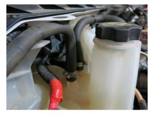
8. Remove coolant tank lower hose and disconnect level sensor plug (three 10 mm nuts).
