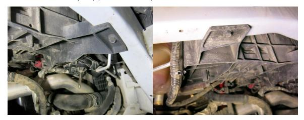
7. Remove the coolant tank top lines.
