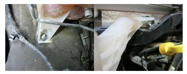
10. Remove the coolant tank.
