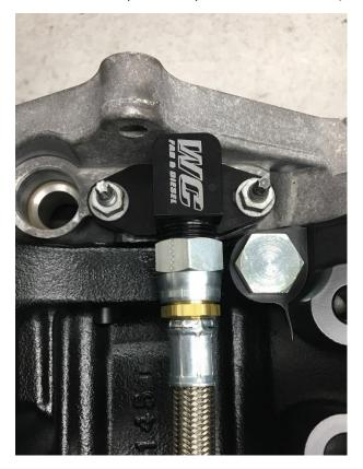
6. On 2001-2010 models, the OEM turbo feed line is in the valley center of the block. You will install the supplied m12 fitting here to block this port.
