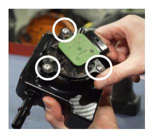
If you are planning on using the pressure sensor port on the filter base, remove the plug and install the sensor now. If you are not planning on using a pressure sensor, make sure the supplied plug is installed (item #5). *Use thread sealant on the plug to prevent leaks.*
