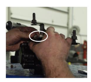
8. Install the new WCFab filter base and mounting bracket onto the vehicle in the OEM location. Slide the assembly over into the slots. Secure the 3 nuts and make sure they are tight.
