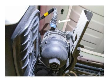
To unseat the blue locking tab, FIRST push the body of the connector toward the filter housing to release pressure on the locking tab. SECOND, squeeze either side of the top of the blue locking tab. With the tabs squeezed, the quick disconnect can be pulled from the housing.
