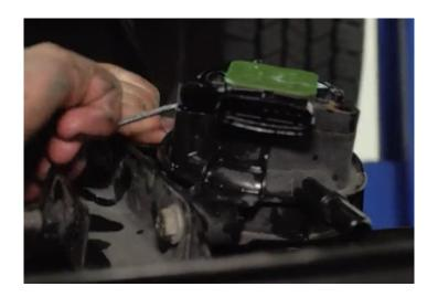
Remove and discard the OEM O-rings on the fuel heater. Install the new O-rings included with the kit and lubricate the O-rings with assembly lube or clean diesel fuel. Using the new hardware supplied in the kit, reinstall the heater on the new WCFab filter base. It can only be installed one way.
