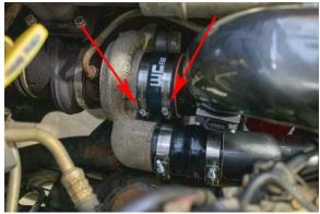
12. Tighten intake clamp and re-check turbo side clamp.
