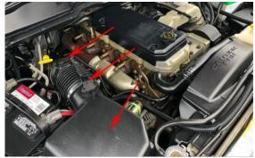
5. Remove OEM air Intake. Remove MAF sensor and save for later reinstallation.
