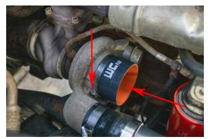
6. Install supplied 4" Straight Boot on turbocharger inlet with Clamps oriented upwards. Tighten Turbo side clamp. Leave intake side clamp loose.
