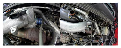
8. Remove factory crossover pipe and install MAP sensor in new WCFab cross over pipe.
