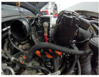
5. Remove the passenger side intercooler pipe connection at the intake air valve by rotating the locking ring at the intake air valve counterclockwise slightly while pulling the pipe towards the front of the truck with a flat head screwdriver for assistance. Note: The intercooler pipe will rotate out of the way. No need to remove lower connection for the installation of this part.
