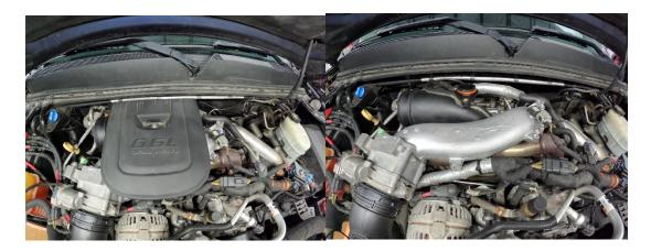
4. Remove the MAP sensor connector, intake air valve connector, grid heater connectors and battery cable from grid heater using a 10 mm socket.
