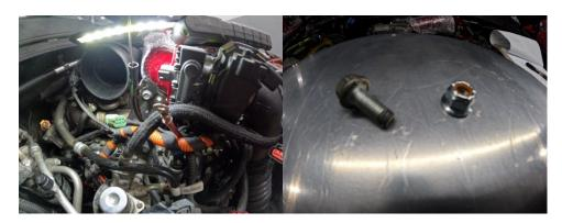
19. Attach connectors for intake air valve, grid heater and battery cable for grid heater.
