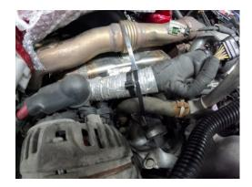
18. Install one bolt previously removed from the dipstick tube bracket and supplied locking
