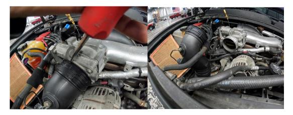
6. Loosen the four 10mm bolts on the intake air valve and remove from the truck.
