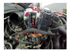
20. Install air box lid and MAF connectors as well as intercooler temp sensor connector.
