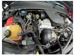
3. Remove the resonator from the turbo inlet by removing two 10mm bolts on resonator.
