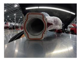
10. Set crossover pipe into place and start one bolt into the engine side (DO NOT TIGHTEN
