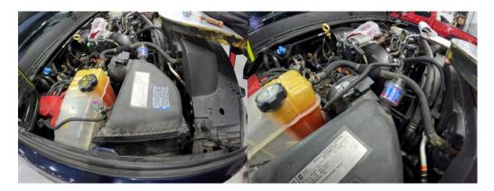
21. Reinstall intake tube and air box lid.
