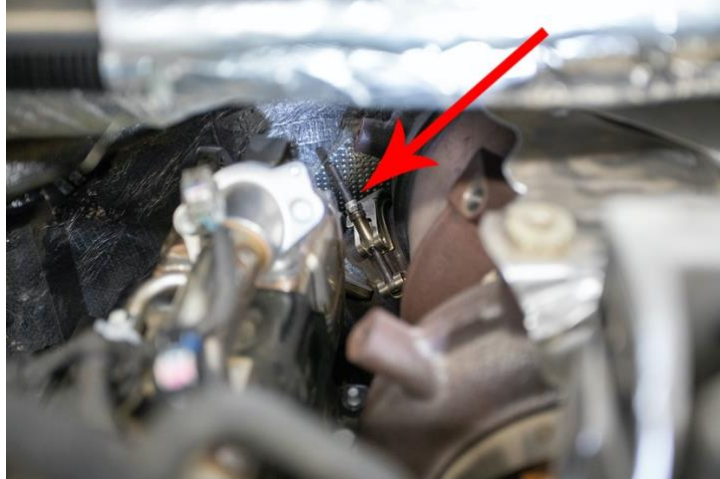
27. Tighten V-band clamp to hold pipe in place but do not fully tighten.
