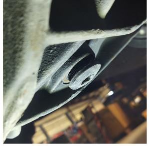
3. Remove the brake line brackets and push them up out of the way on top of the differential. The hardware will be reused for install of bracket.
