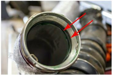
18. Install 2 o-rings, dry, in lower grooves as shown. Once o-rings are fully seated, apply transmission assembly lube (such as Trans-Jel or Dr. Tranny's Assemblee Goo) to inside of pipe connection, o-rings, and intercooler outlet to help prevent damage during install. Avoid using petroleum or other synthetic lubricants which may damage o-ring seals.
