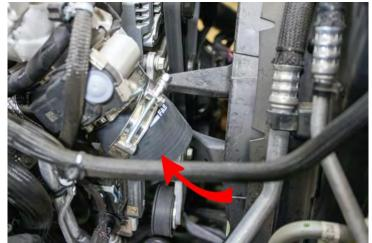
20. Install top boot and clamps onto the engine intake side and leave loose.
