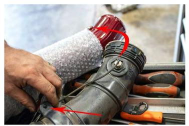
17. Swap charge air temp sensor from OEM intercooler pipe to your new 3.5" intercooler pipe using a pry tool to remove wire harness clip and a 14 mm wrench. Liquid Teflon thread sealant is recommended on the sensor during re-installation for a leak free seal.
