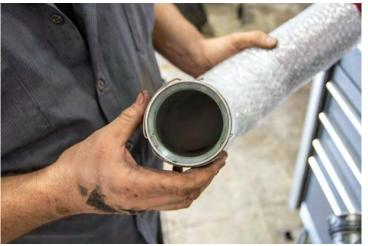
16. Transfer clip ring to the new intercooler pipe assembly. NOTE: Pay close attention to orientation of clip ring on the new pipe as it will only properly engage the pipe and intercooler assembly one way. One groove in the pipe is smaller than the other two. Reference image above to make sure your ring position matches the mounting shown.
