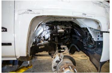
4. Remove the passenger side wheel/tire and inner fender liner.
