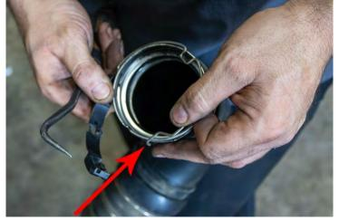
15. Remove clip ring from lower OEM Intercooler pipe connection using a pick or flat blade screwdriver.
