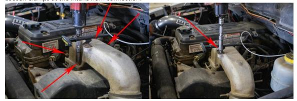
4. Using a 10mm socket and extension, remove intake horn bolts and disconnect dipstick support bracket.
