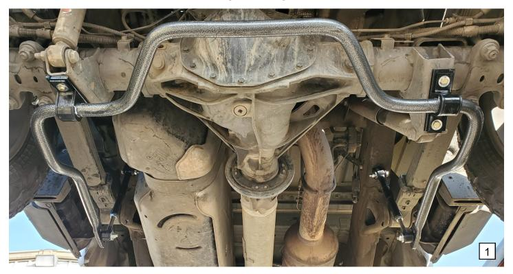
SAFETY: BEFORE STARTING YOUR INSTALLATION, PARK YOUR VEHICLE ON A FLAT LEVEL SURFACE, SET THE PARKING BRAKE, CHOCK THE FRONT TIRES.
