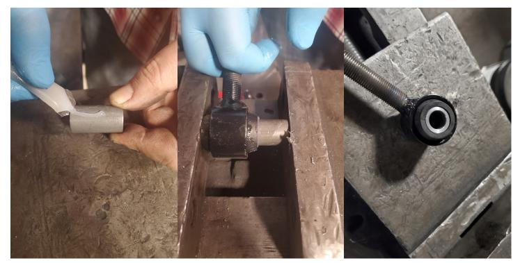
Next, take the bushing sleeve and lube the Place the end-link with the hourglass outside of it. Spread the lube around evenly.
