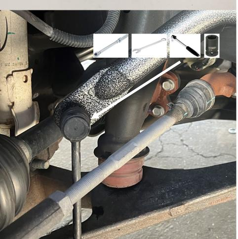
Step 6: Attach upper End-Link Bolt
