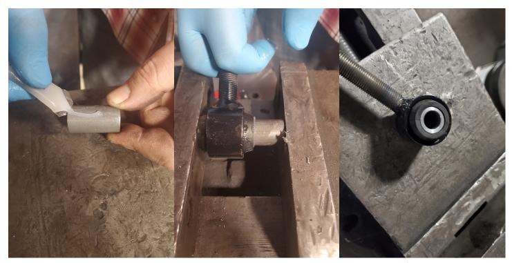
Next, take the bushing sleeve and lube the Place the end-link with the hourglass outside of it. Spread the lube around evenly.
