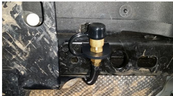
Figure 22 - Air Coupler Mounted To Bumper
