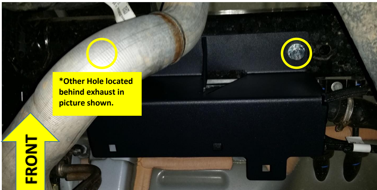
Figure 13 - JL-204 Adapter Bracket Bolted in Place
