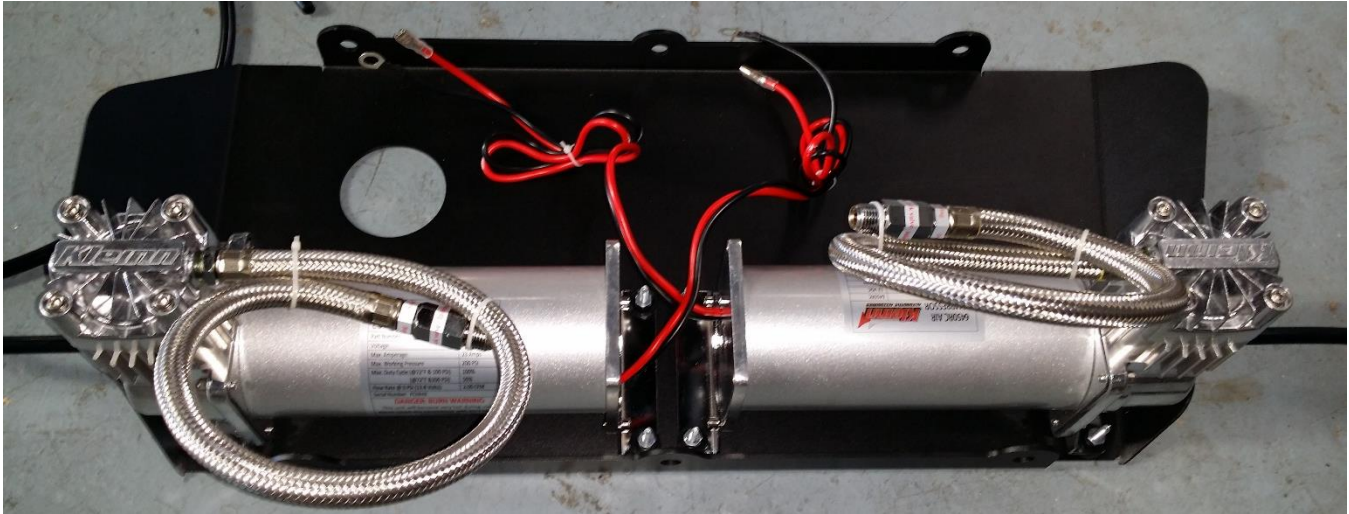
Figure 3 - Compressor Mounted onto JK-101 **JK6450 Upgrade Shown
