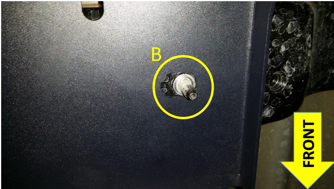
Figure 18 – Ground Strap Nut removed; JK-201 Tank Bracket shown in place
