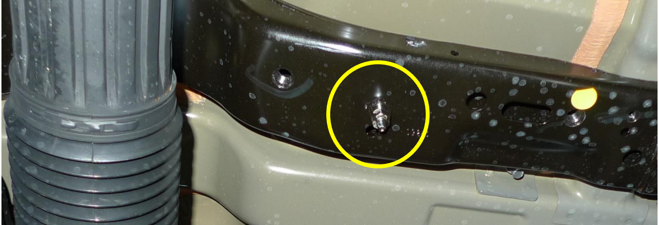
Figure 14 – JLU Middle Crossmember & Ground Strap Mounting Point
