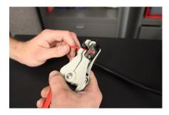
**B.** Place wire from 46044 and WH-1006-3 into butt connector. Using crimping tool connect 46044 and WH-1006-3 with butt connector. Install 46260 to 46044 bottom slot (opening that is near the spade).
