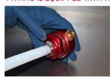
I. Place the BHF-1002 bulkhead fitting on the tank with enough clearance for the fuel line and fittings. Keep in mind the bulkhead must also clear the bottom of the bed support structure.
