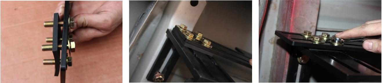
**H.** Once secure use 3-1 3/4 bolts and 3-WA-1001D spacers to mount the pump to the bracket.
