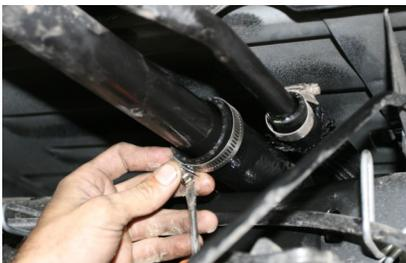
**C.** Disconnect factory suction and return lines (refer to diagram at the beginning of step 2).
