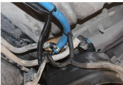
**Note: Secure all fuel lines with cable ties. Cable ties are an economical way to prevent the possibility of problems occurring! The factory suction line can be capped off or removed from the truck. The openings on the filter and tank will need to be capped off to keep debris from getting into lines or canister.**
