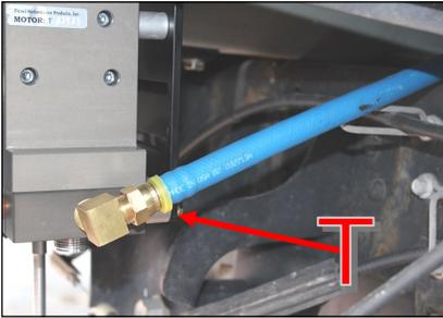
**NOTE: Hose clamps are not recommended for push lock fittings. They will hold up to 300psi! Use oil on fittings and inside fuel line when installing Push-Lok fittings**
