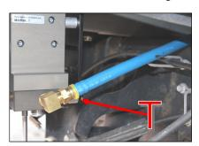
NOTE: Hose clamps are not recommended for push lock fittings. They will hold up to 300psi! Use oil on fittings and inside fuel line when installing Push-Lok fittings
