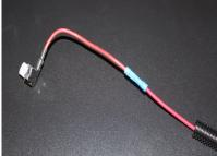
**C.** Crimp the ring terminals to the red and green wires of the WH-1006-3 Wire Harness. Attach red wire to the positive terminal of the battery and the green terminal to the negative terminal. The use of a corrosion preventative on electrical connections is recommended.
