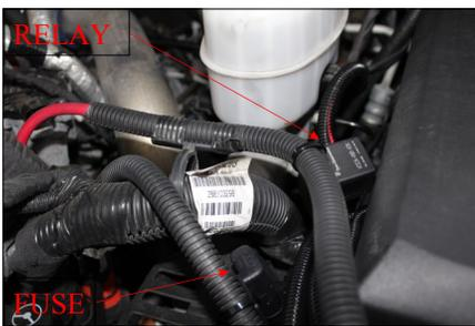
**E.** Route the extension to the engine bay fuse panel. Remove a fuse (maximum of 10A) that is “hot” when the key is on. Example: #54 or #55. **Use a test probe to locate the “hot side” of the circuit in the fuse block.** Install the fuse tap into the open location. Install the pulled fuse into the open space on the fuse tap. Disconnect the vehicles’ battery and continue installation.
