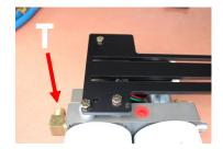
**C.** Assemble PFB-2002C and RS-2001C RS will make contact with bed channel when assembled correctly. Insert the PFB-2002C assembly in to bed channel align the nut with the opening on the channel.
