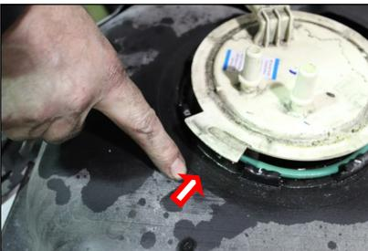
G. Once the lock ring is removed, carefully remove pick up module from fuel tank without bending fuel level arm.
