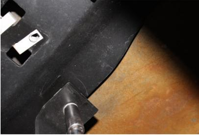
E. Clean the fuel module area then remove the lock ring on the top of the fuel tank. **This is spring loaded, so, holding it down while removing the ring will prevent the sending unit from popping up and possibly causing damage.**
