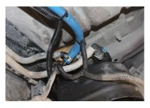
Note: Secure all fuel lines with cable ties. Cable ties are an economical way to prevent the possibility of problems occurring! The factory suction line can be capped off or removed from the truck. The openings on the filter and tank will need to be capped off to keep debris from getting into lines or canister.
