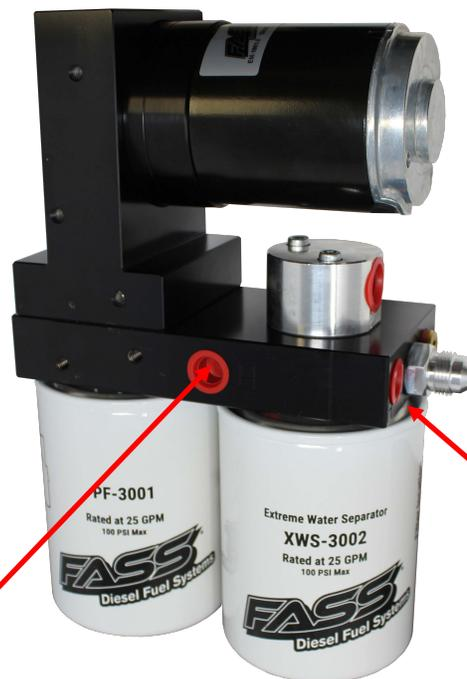
**Note: The Red Plastic Plugs located in the "H" ports can stay in place fuel will not flow through these ports. Coolant can be plumbed into these ports to heat the fuel in the Winter months.**
