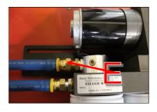
**D.** Disconnect factory fuel supply line on rear of factory Ford lift pump, and connect FASS hose using fitting A624C56-55-05 and HC-1001.
