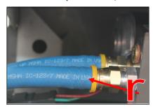
**C.** Insert PL-1005 into remaining fuel line using oil. Attach fuel line to the 'E' port of the FASS system. Torque to 18 ft./lbs. Route this line to the engine side of the factory lift pump. Do not cut at this time.
