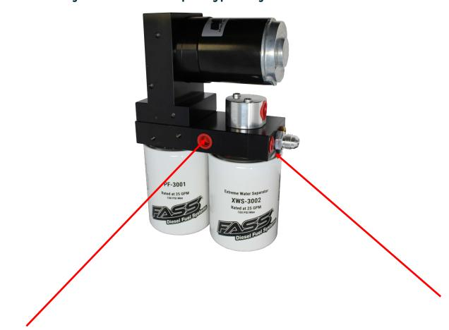
Note: The Red Plastic Plugs located in the "H" ports can stay in place fuel will not flow through these ports. Coolant can be plumbed into these ports to heat the fuel in the Winter months.
