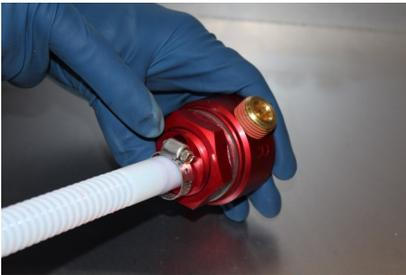
I. Place the BHF-1002 bulkhead fitting on the tank with enough clearance for the fuel line and fittings. **Keep in mind the bulkhead must also clear the bottom of the bed support structure.**
