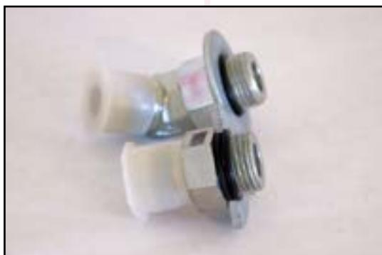
8. Now Remove the old radiator to transmission cooler line and replace it with the new line (straight fitting on one end, and a 90° fitting on the other end). Once again leave all the hose fittings loose until the final alignment (after all hoses are installed).
