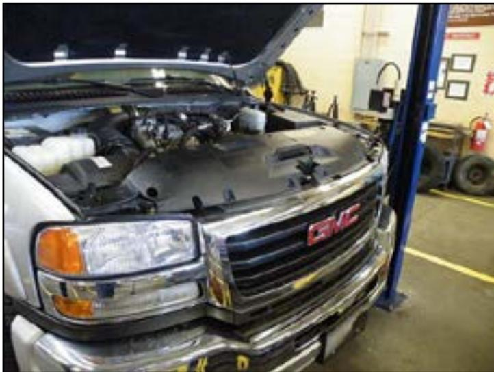
2. Next remove the bolt for the grille. Then pop the two outer snaps on the outer ends of the grille (both sides) and then the four main snaps. Then Lift the grille out.
