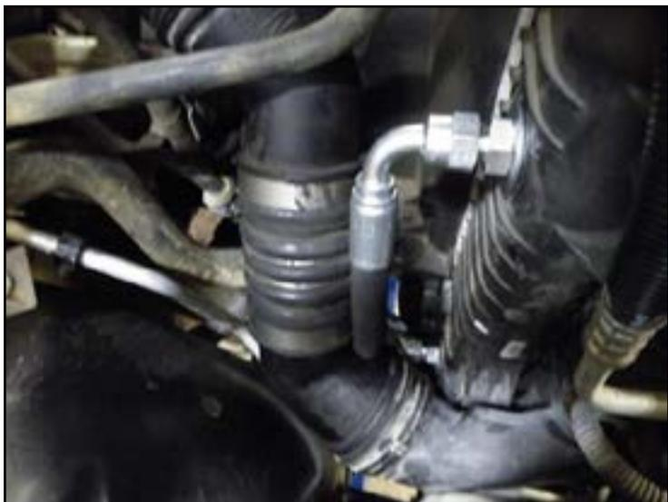
9. After all the lines are aligned, tighten all the fittings except the upper radiator fitting. Remember to use a wrench to counter torque your tightening on both transmission cooler fittings so you dont bend or distort it.
