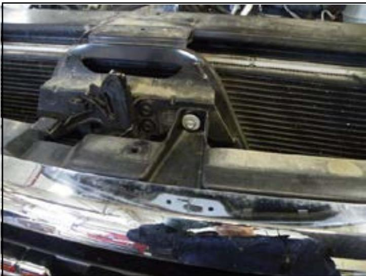
3. Remove the air filter box, the plate under it, the bracket under that, and the CAC (Charged Air Cooler/Intercooler) hose on the discharge side of the CAC so you will have access to the hoses and fittings going into the radiator and transmission cooler.
