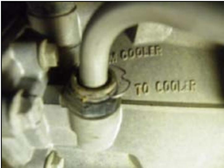
5. Next remove the lines from the Transmission Cooler and the threaded fittings. Be careful when loosening the fittings, as the aluminum cooler is very soft and a counter torque is necessary to prevent twisting the ends of the cooler. Also there could be additional fluid drainage from the fittings at the cooler, and the other ends of the transmission. The fittings you use in the transmission cooler are the 90° short fittings.
