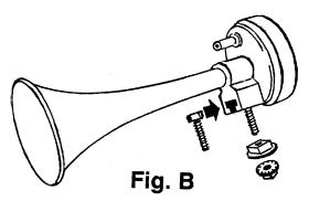
3. **IMPORTANT:** Mount trumpets with the open ends facing down. This will prevent water from entering into the trumpets and compressor. **Water damage to the horn's component parts is not covered by our factory warranty.**
