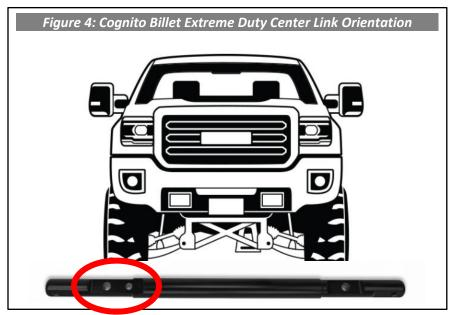
**8.** Install the Cognito Billet Extreme Duty Center Link onto the pitman and idler arms with the steering stabilizer hole towards the passenger side of the vehicle. Reuse the factory lock nuts and torque to 70-ft-lbs.
