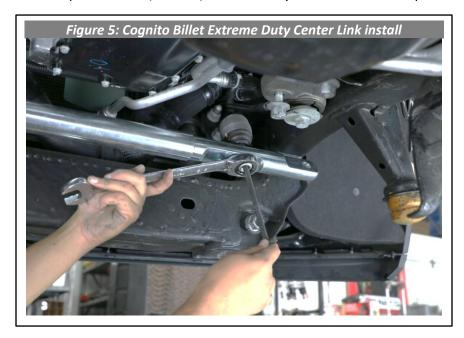
**9.** Remove the nut attached to the pre-assembled Cognito tie rod and insert the tie rod through the center link's tapered hole. Test fit the tie rod assembly. Fasten the nut back onto the tie rod and tighten hand tight.
