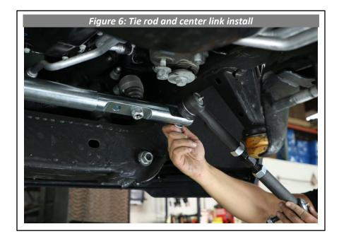
**10.** Wipe down and clean the tapered hole in the spindle where the outer tie rod will connect. Remove the nut attached to the pre-assembled Cognito tie rod and insert the outer tie rod into the tapered spindle hole. Fasten the nut back onto the outer tie rod and tighten hand tight.
