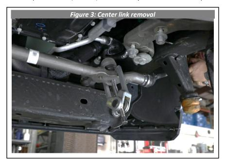
7. Locate the Cognito Billet Extreme Duty Center Link (PN 6529). One side of the center link has one additional hole for the steering stabilizer. This side will be installed towards the passenger side of the vehicle.
