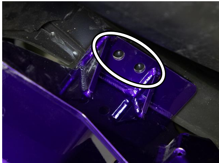
Figure 3: Frame Mounting Hole Marking
