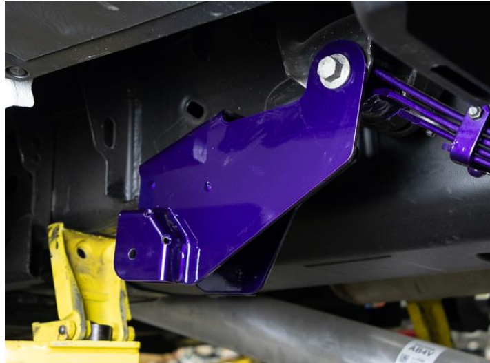
Figure 2: Frame Mount Bracket Installation
