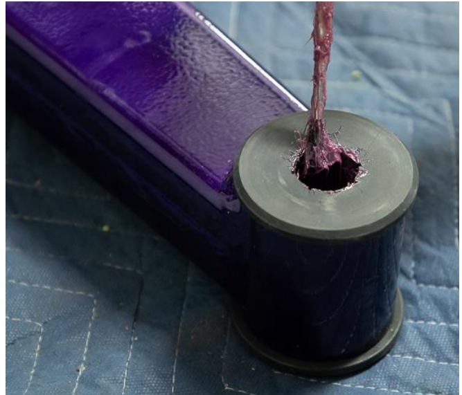
Figure 14: Traction Bar Bushing Grease Application
