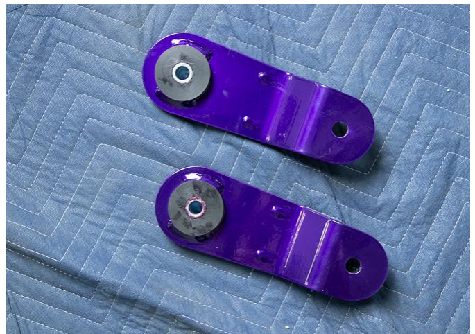
Figure 8: Shackles and Hardware Installation
