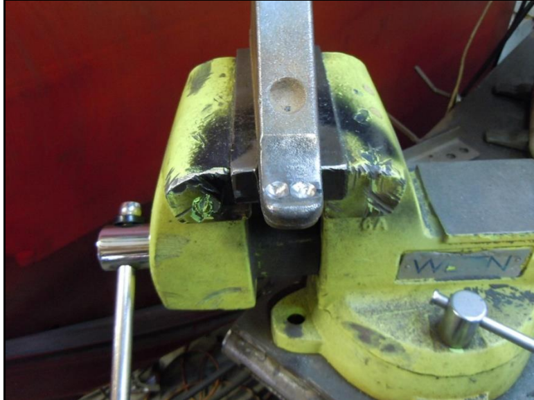
Figure 19: Stock Torsion Key Slotted Pocket Formed.
