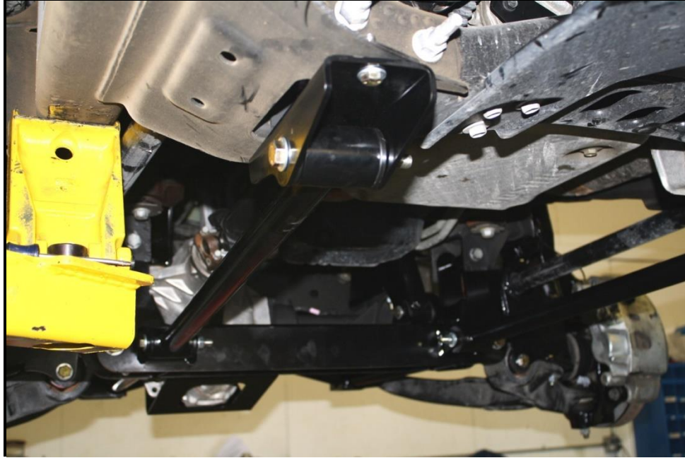
Figure 14: Cognito Compression Strut Installation.
