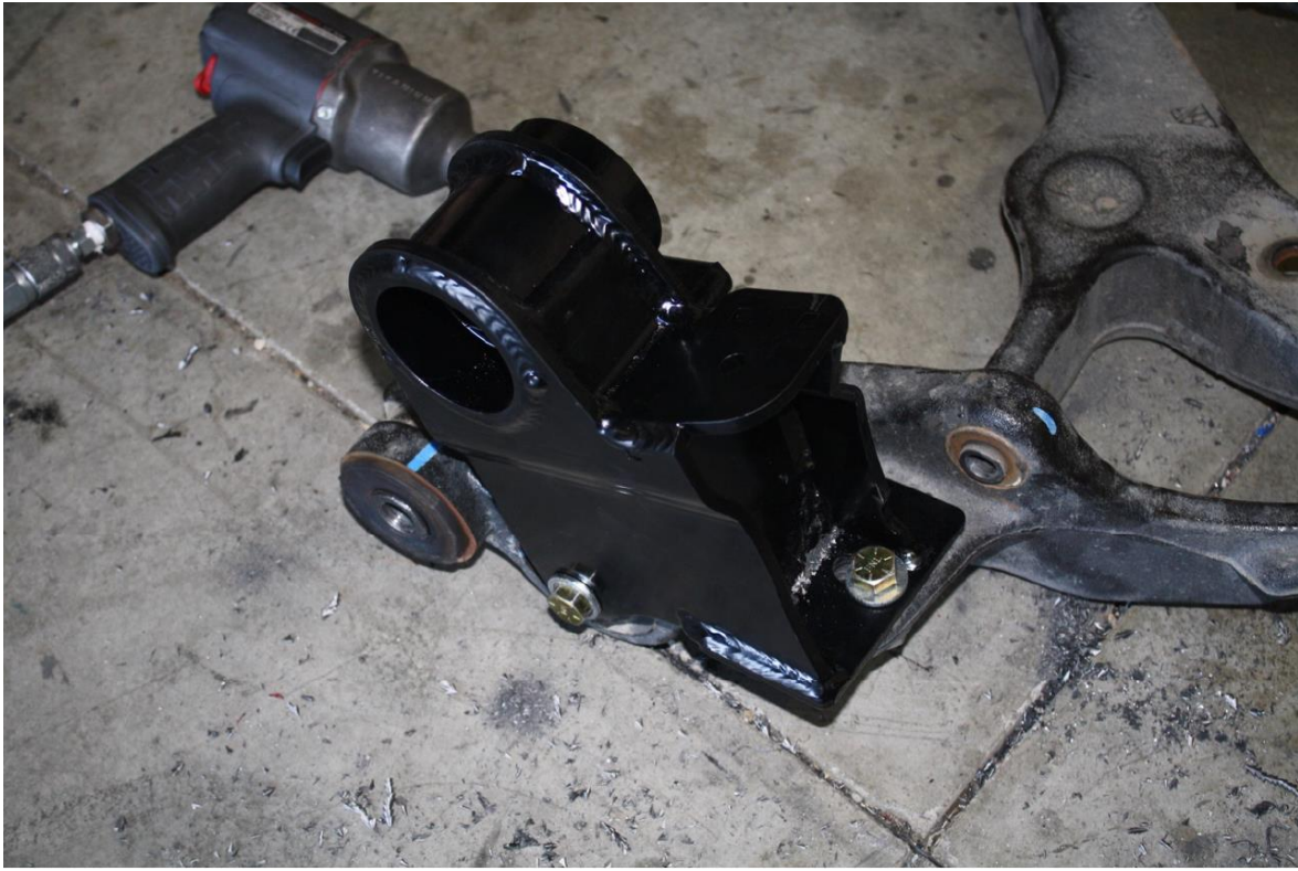
Figure 13: Non-Torsion drop bracket installed on lower control arm. Passenger side shown.
