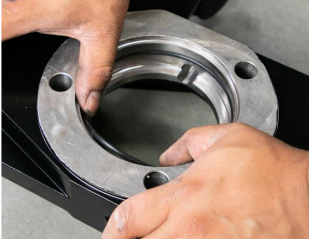
Figure 41c: Installing O-ring in Cognito Spindle
