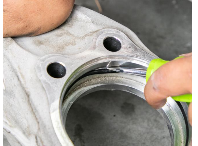
Figure 41b: Removing O-ring from Stock Spindle
