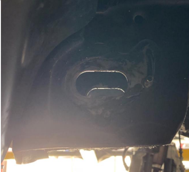
Figure 24g: Driver's Side Front Crossmember, After Trimming
