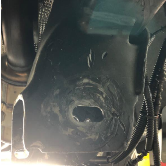
Figure 24e: Driver's Side Rear Crossmember, After Trimming
