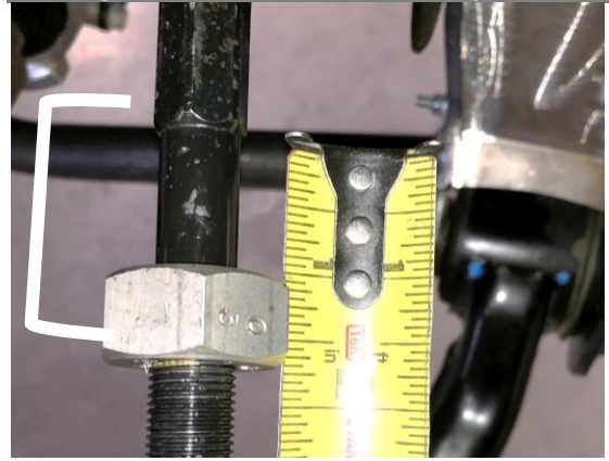
Figure 46b: Measure Position of Die
