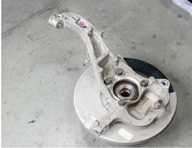
Figure 41a: Hub Installed in Stock Spindle
