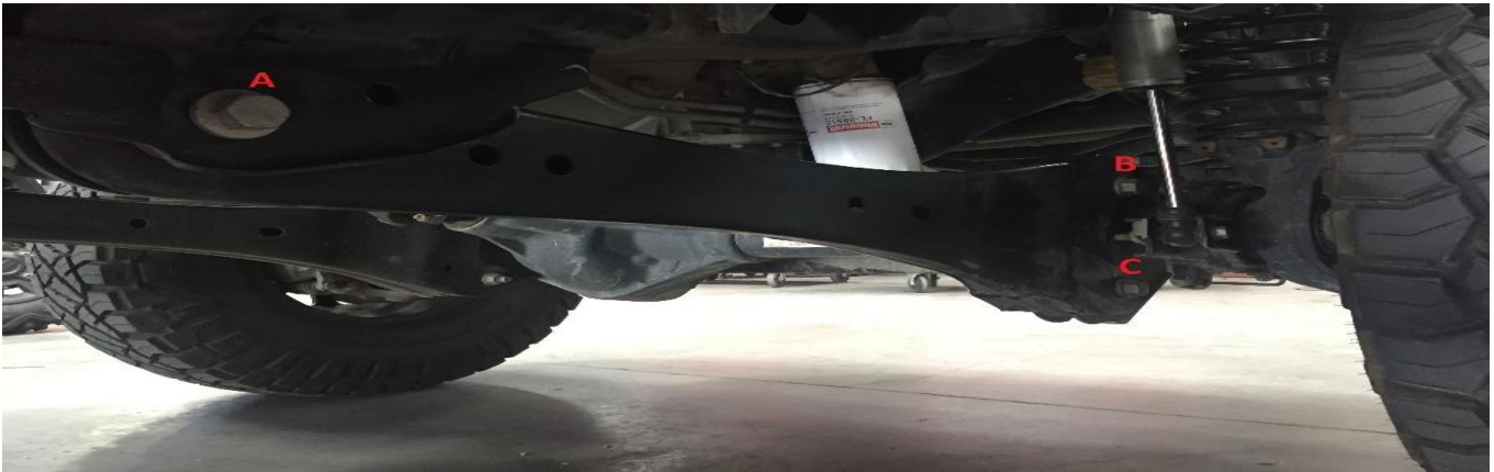
Figure 9: Radius Arm Bolt Locations
