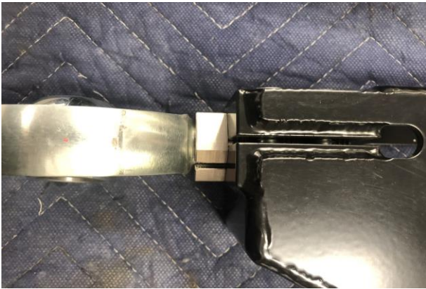
Figure 12: Radius Arm Clevis Adjusting
