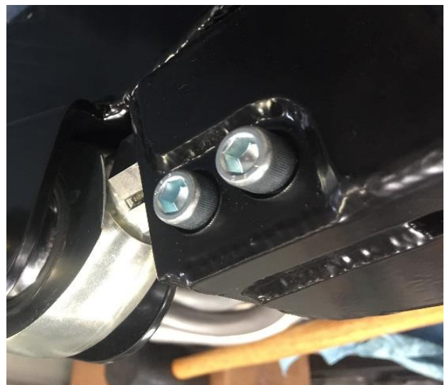
Figure 15: Adjuster Clamp Screws
