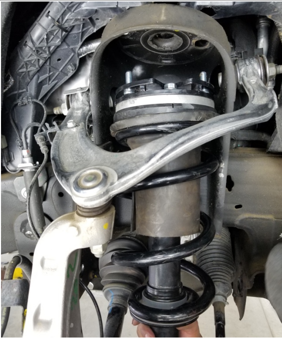
Figure 13: Install Strut With Spacer
