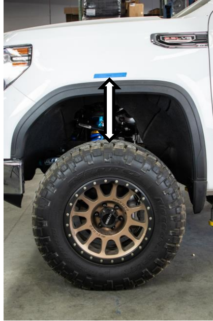
Figure 4: Measuring and Setting Ride Height
