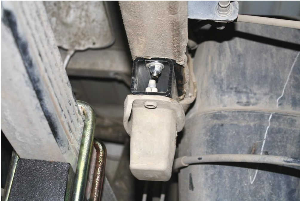
Figure 28: Rear bump stop spacer
