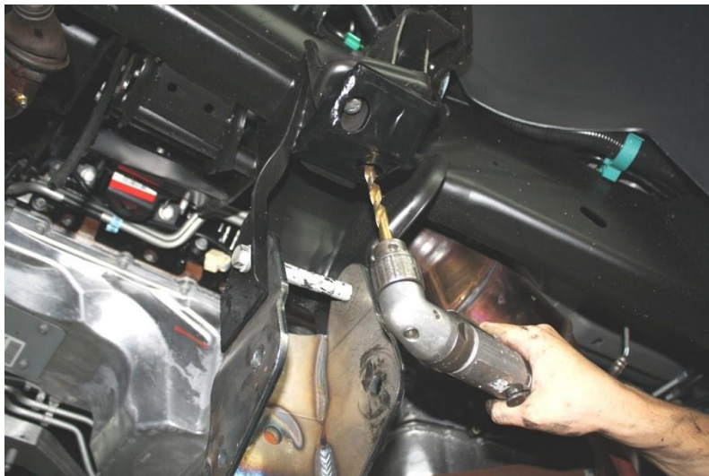
Figure 12: drill mounting hole for bump stop brackets
