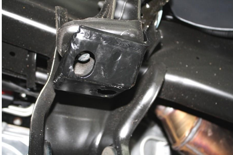
Figure 119: bolt bump bracket to existing hole on bottom
