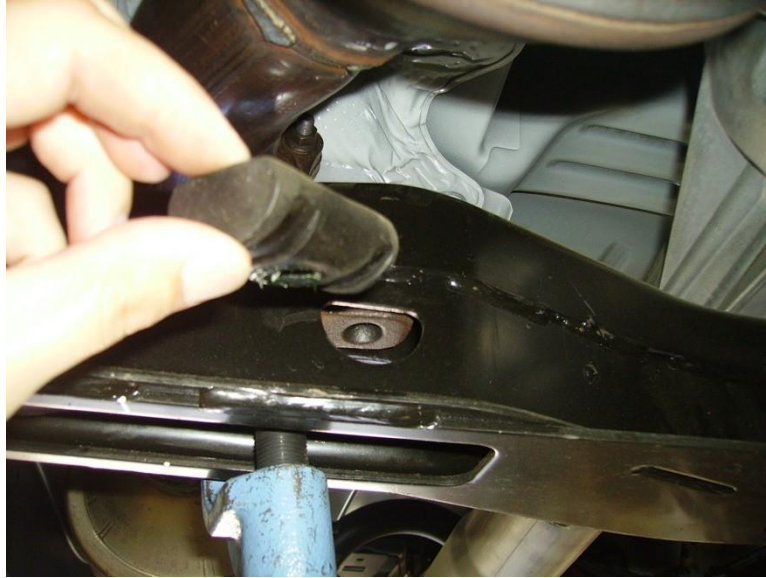
Figure 3: adjuster nut removed
