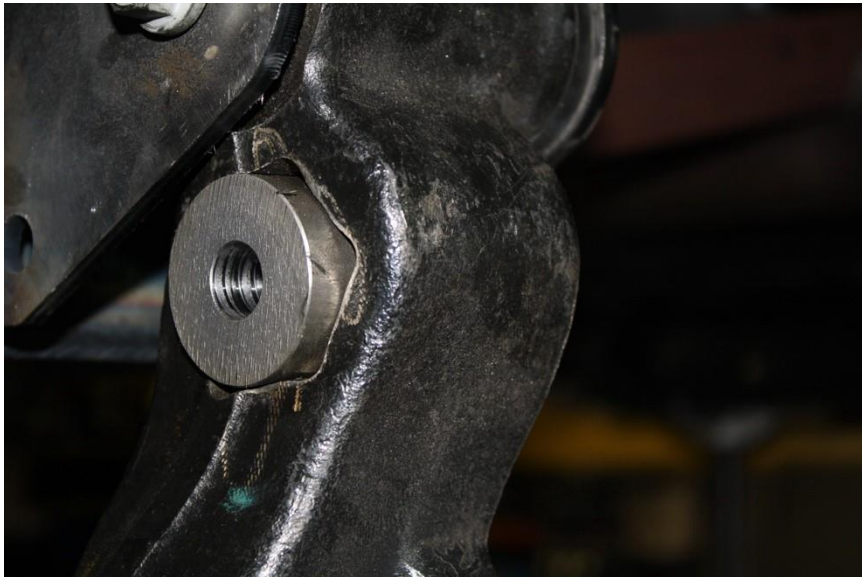
Figure 26: 5388 mandrel inserted into lower control arm.
