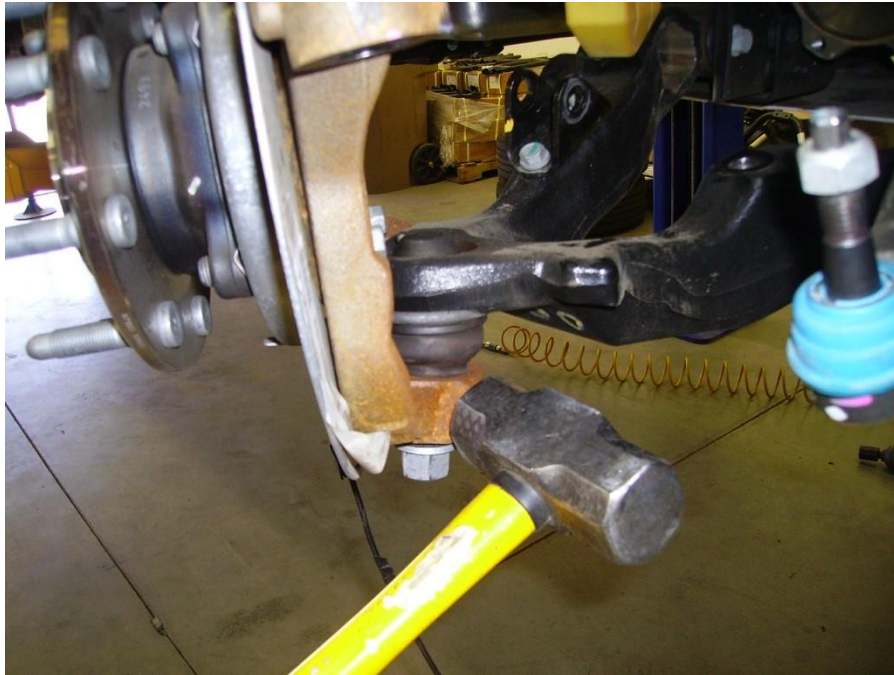
Figure 9: removing lower control arm.
