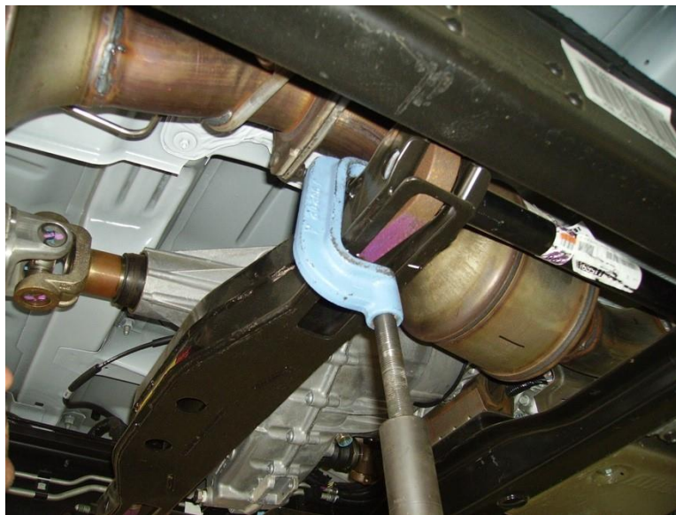
Figure 2: load torsion bar to remove adjuster nut
