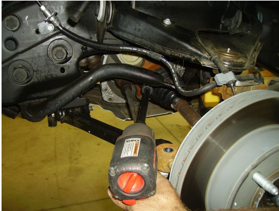
Figure 8: Remove CV axles on 4wd vehicles
