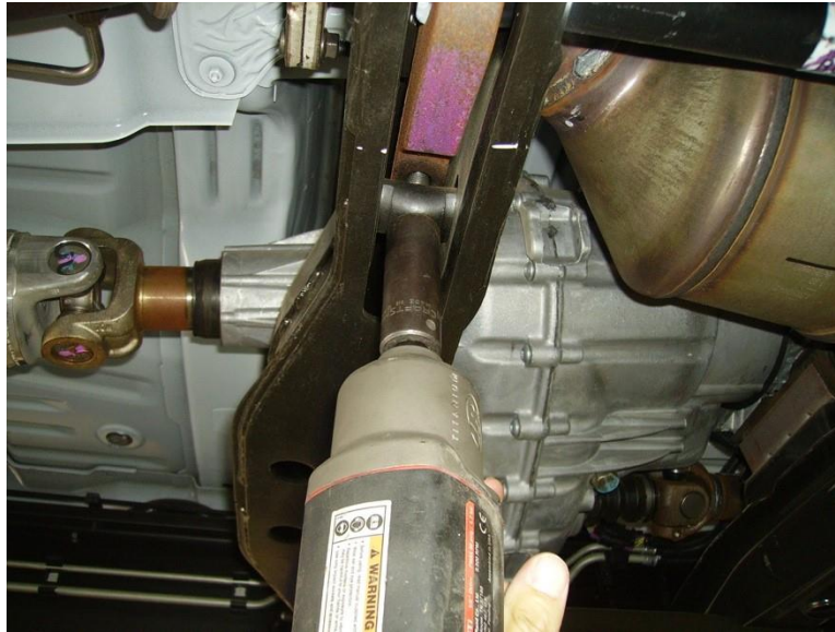
Figure 1: remove torsion bar adjusting bolt
