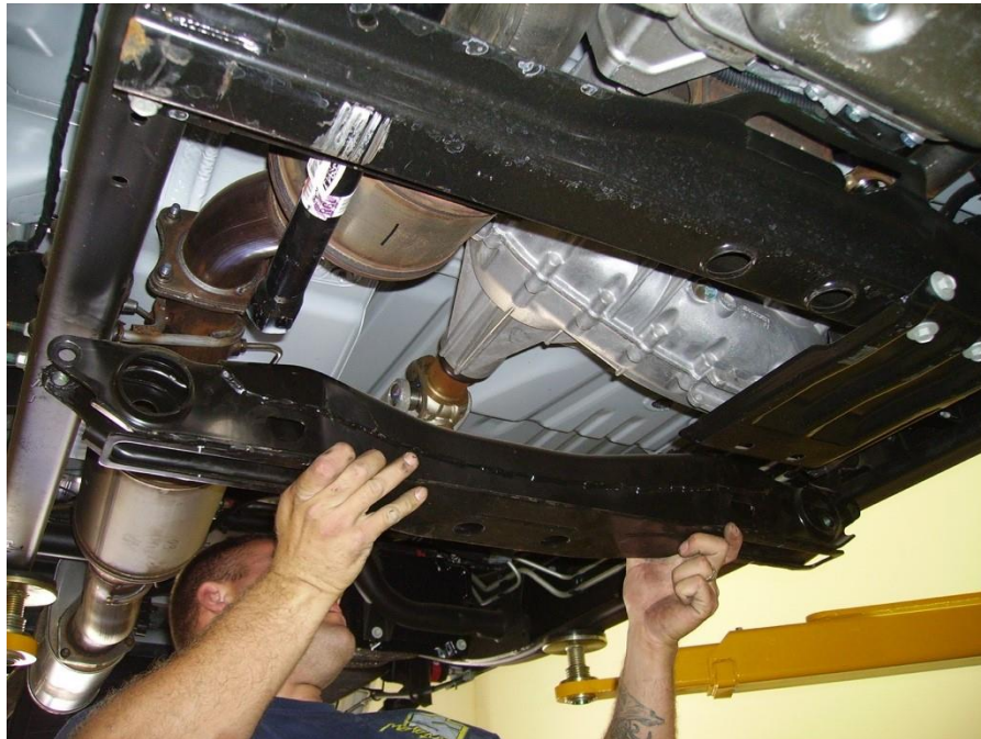
Figure 4: Remove factory torsion bar crossmember
