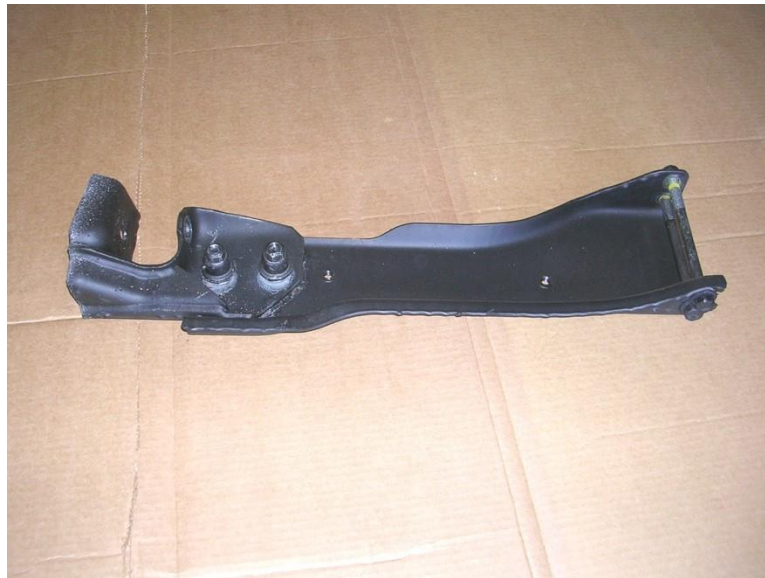
Figure 15: Factory crossmember and frame section removed.
