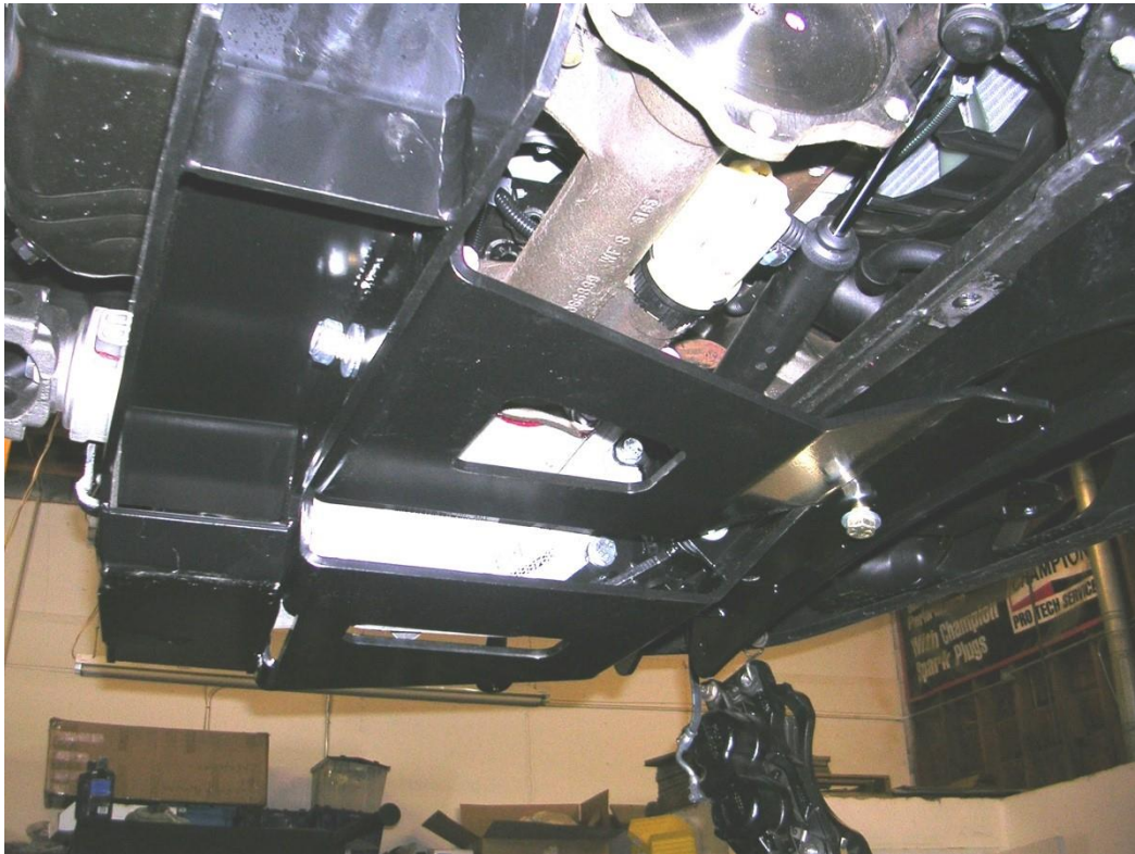
Figure 22: Cognito Skid Plate during installation
