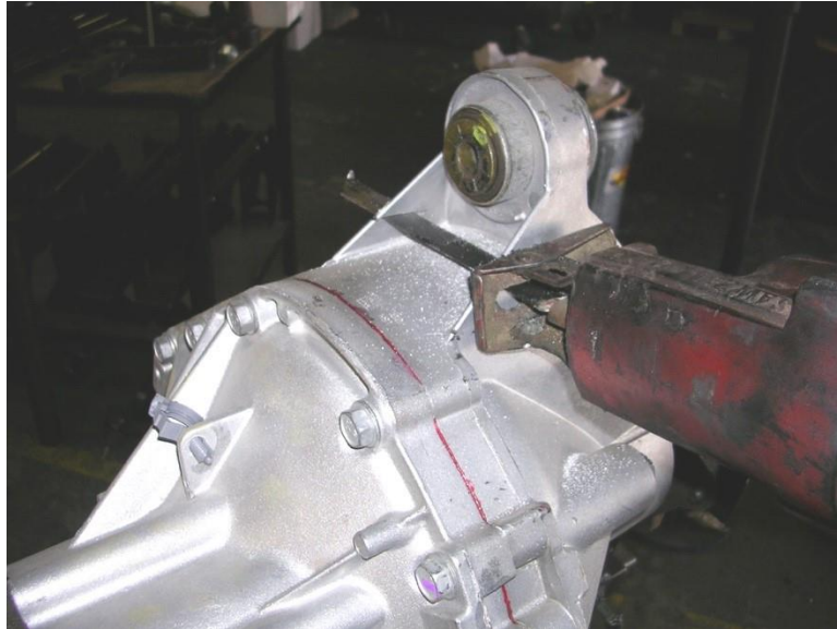
Figure 16: Cutting off mounting ear. Don't worry! We make a replacement if needed later.
