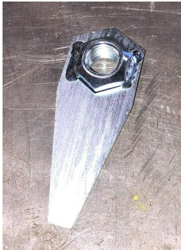
Figure 1. Nut Tab for Axle Side of Track Bar
