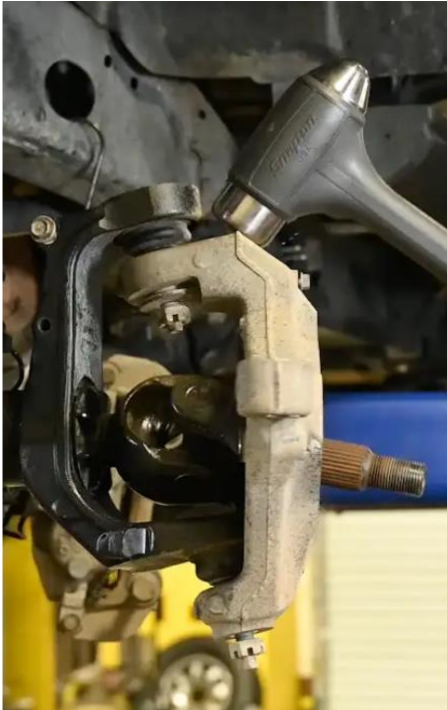
Figure 7. Separating the Upper Ball Joint
