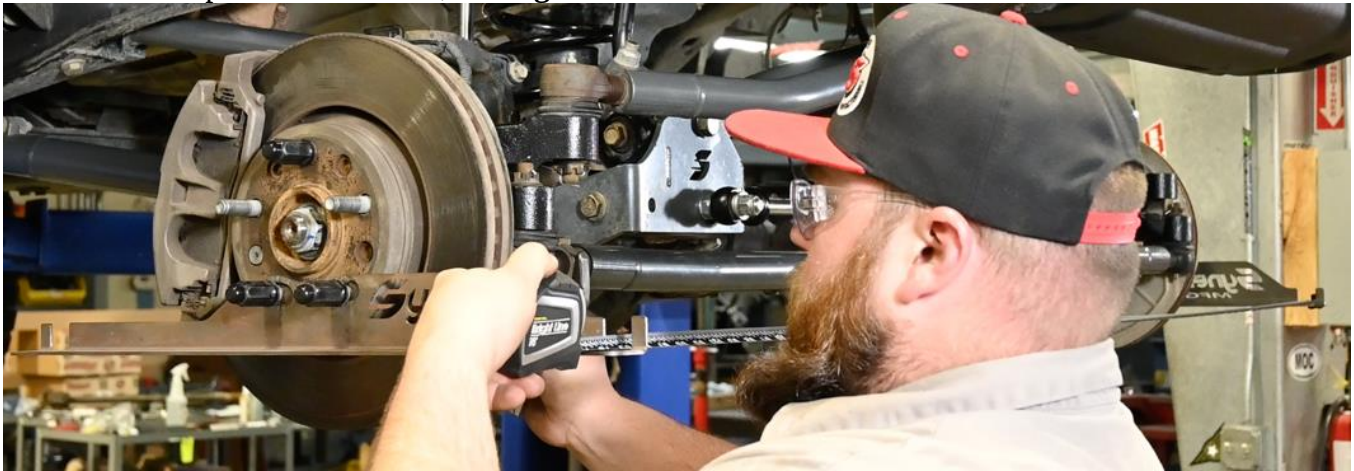
Figure 10. Adjusting Toe with Synergy Alignment Plates
