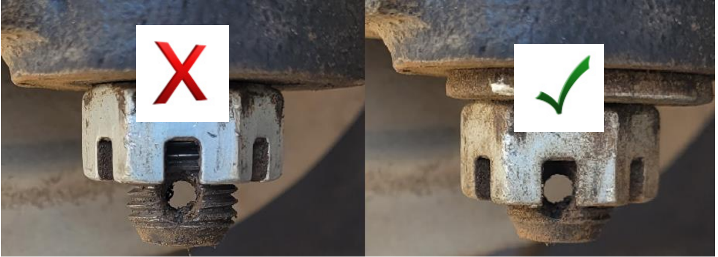
Figure 8. Cotter Pin Alignment on Lower Ball Joint
