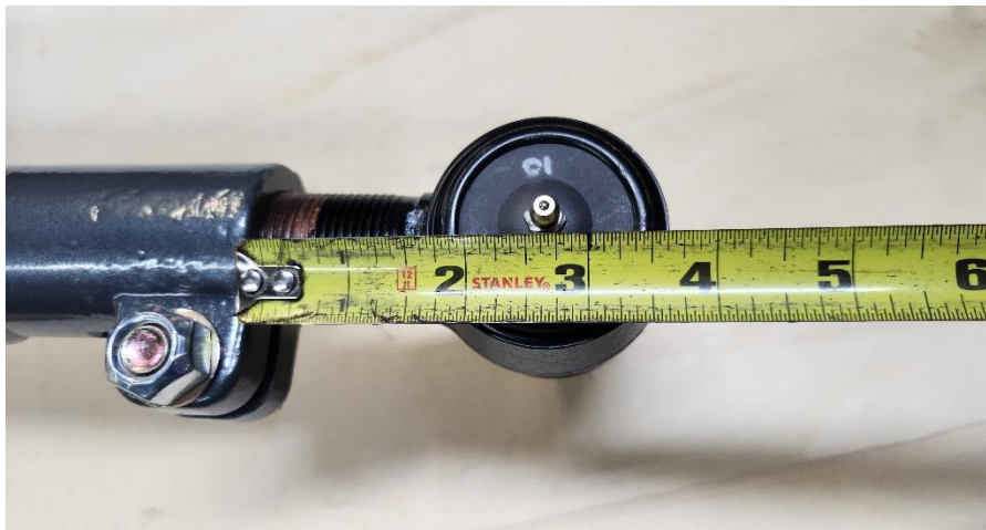
Figure 5. Maximum Length on Non-Double Adjuster (Pass) Side
