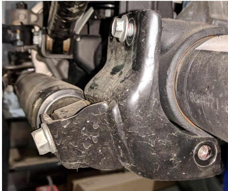
Figure 3. Removing Axle Side Steering Stabilizer Bracket
