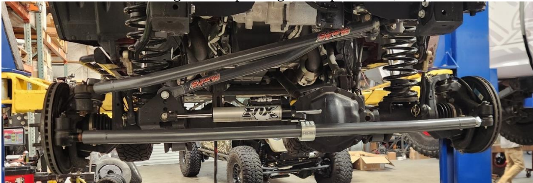
Figure 7. Tie Rod Correctly Oriented, Pinch Bolts Back
