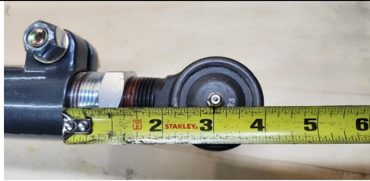
Figure 6. Maximum Length on Double Adjuster (Driver) Side
