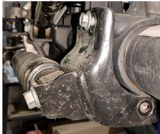
Figure 3. Removing Axle Side Steering Stabilizer Bracket
