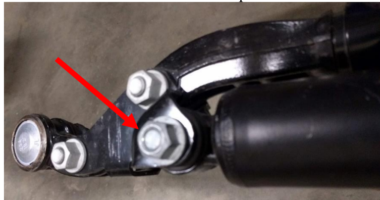
Figure 1. Removing Stabilizer Nut from Underside of Tie Rod
