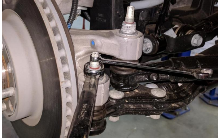
Figure 2. Using Two Wrenches to Loosen Tie Rod End Nuts
