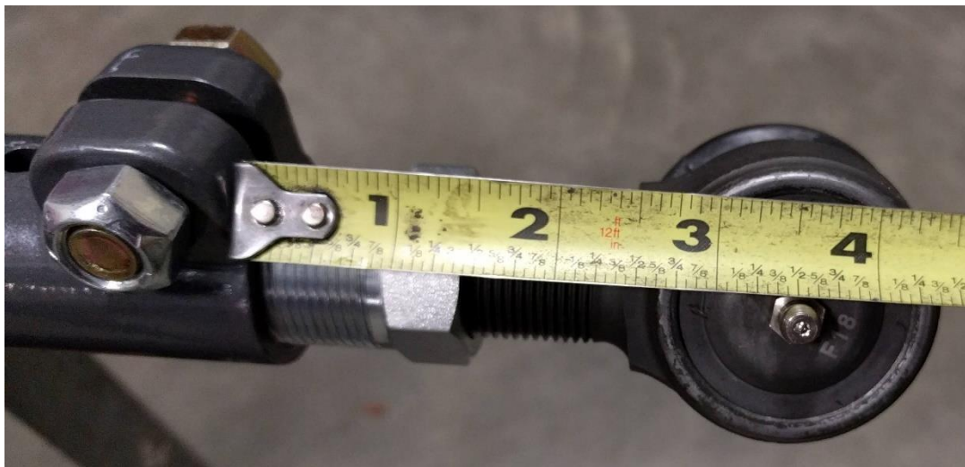
Figure 6. Maximum Length on Double Adjuster (Passenger) Side
