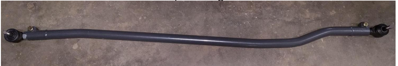
Figure 4. Synergy MFG Tie Rod Shown From Above
