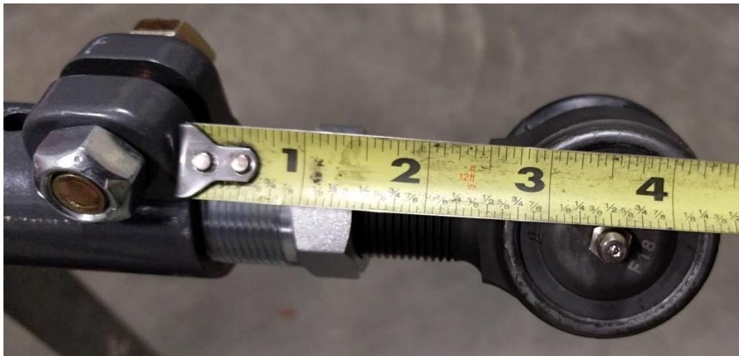
Figure 6. Maximum Length on Double Adjuster (Passenger) Side
