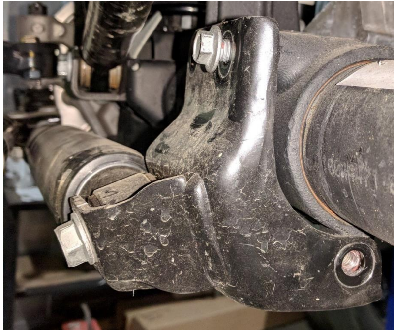
Figure 3. Removing Axle Side Steering Stabilizer Bracket
