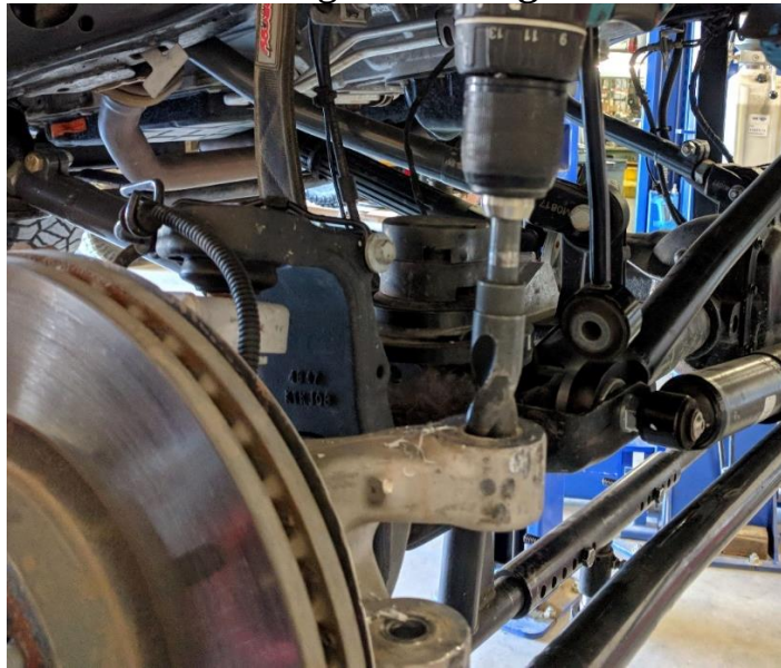
Figure 3. Drilling out Steering Knuckle
