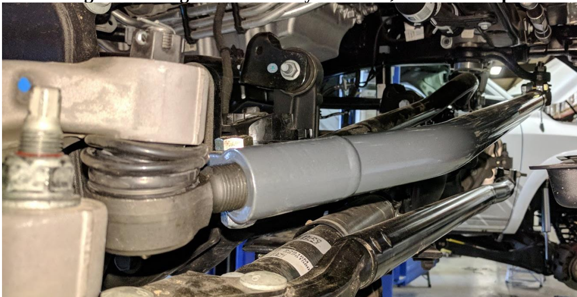
Figure 8. Drag Link Correctly Oriented, Pinch Bolt Back, Bend Forward
