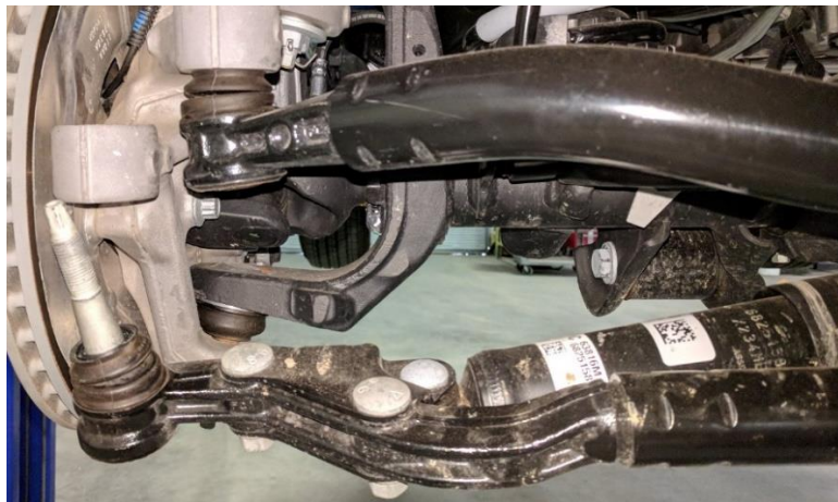
Figure 2. Tie Rod Removed From Knuckle
