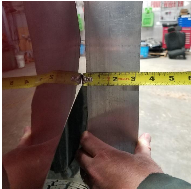
Figure 11. Measuring the Distance from the Tire Face to the Fender.
