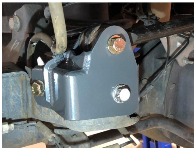
Figure 8. Installed Track Bar Relocation Bracket with Factory Rear Track Bar.
