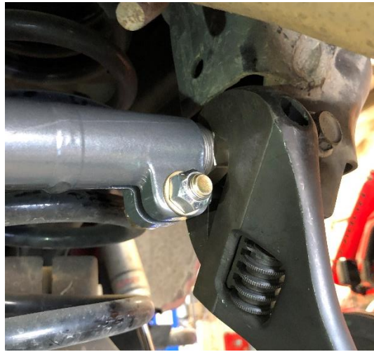
Figure 10. Adjusting the Rear Track Bar to Align the Frame Side Bolt.
