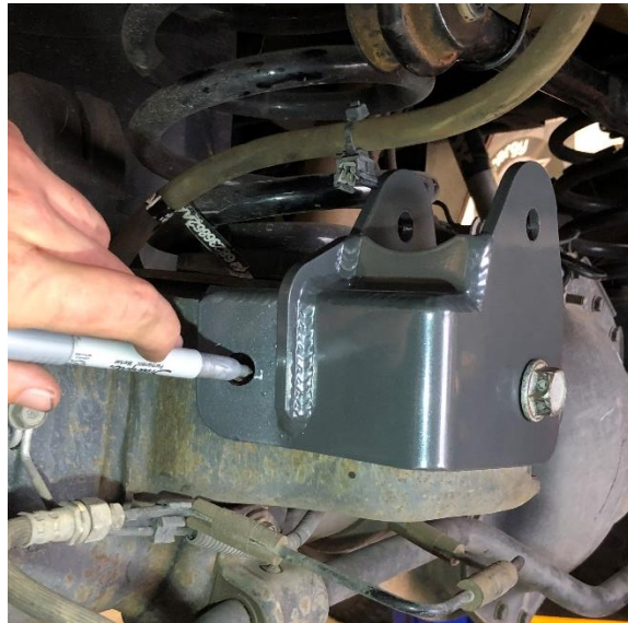
Figure 6. Marking the Factory Bracket for Drilling.
