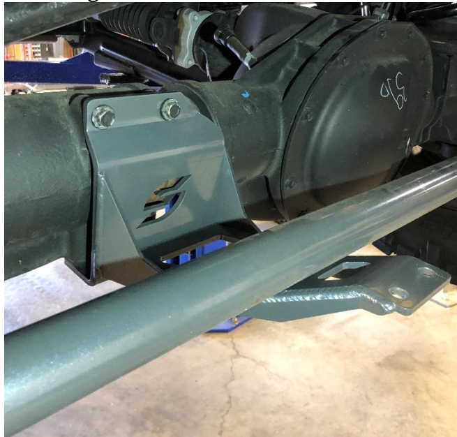
Figure 3. Dual Stabilizer Bracket Indexed on the Differential Housing
