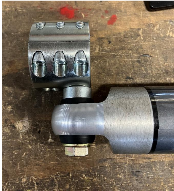
Figure 9. 4050-75 Clamp Installed on Steering Stabilizer with Spacer.
