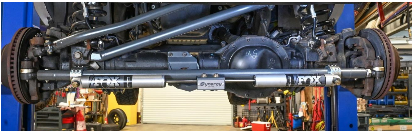
Figure 10. Dual Steering Stabilizers Installed on Dual Stabilizer Bracket
