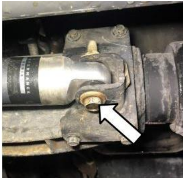
Figure 1. Stabilizer Bolt to be Removed
