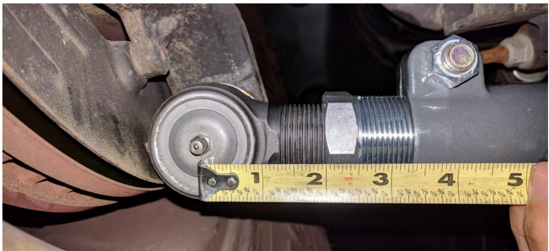
Figure 9. Double Adjuster Tie Rod End Max Extension
