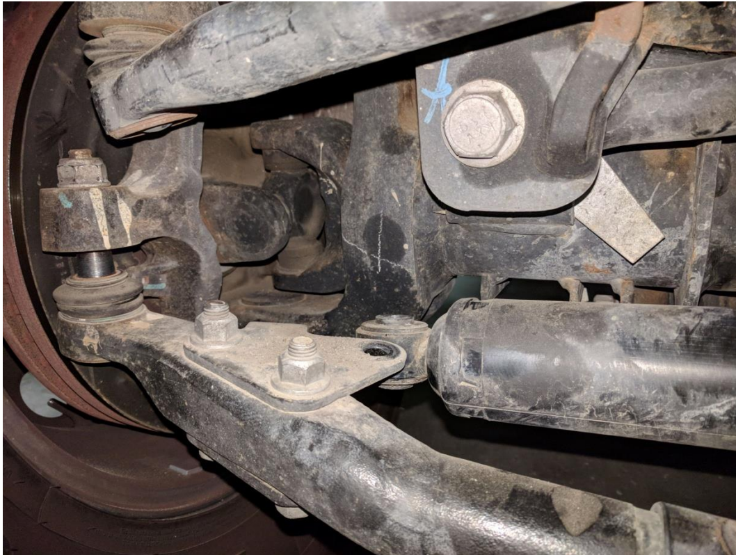
Figure 1. Steering Stabilizer Removed From Stock Tie Rod
