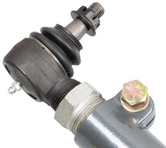
Figure 3. Double Adjuster Side of Tie Rod
