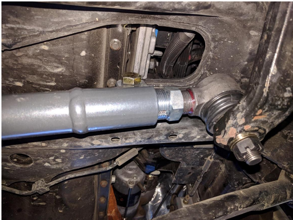
Figure 3. Double Adjuster End of Drag Link at Pitman Arm
