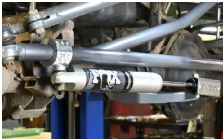
Figure 6. Correctly Installed Stabilizer
