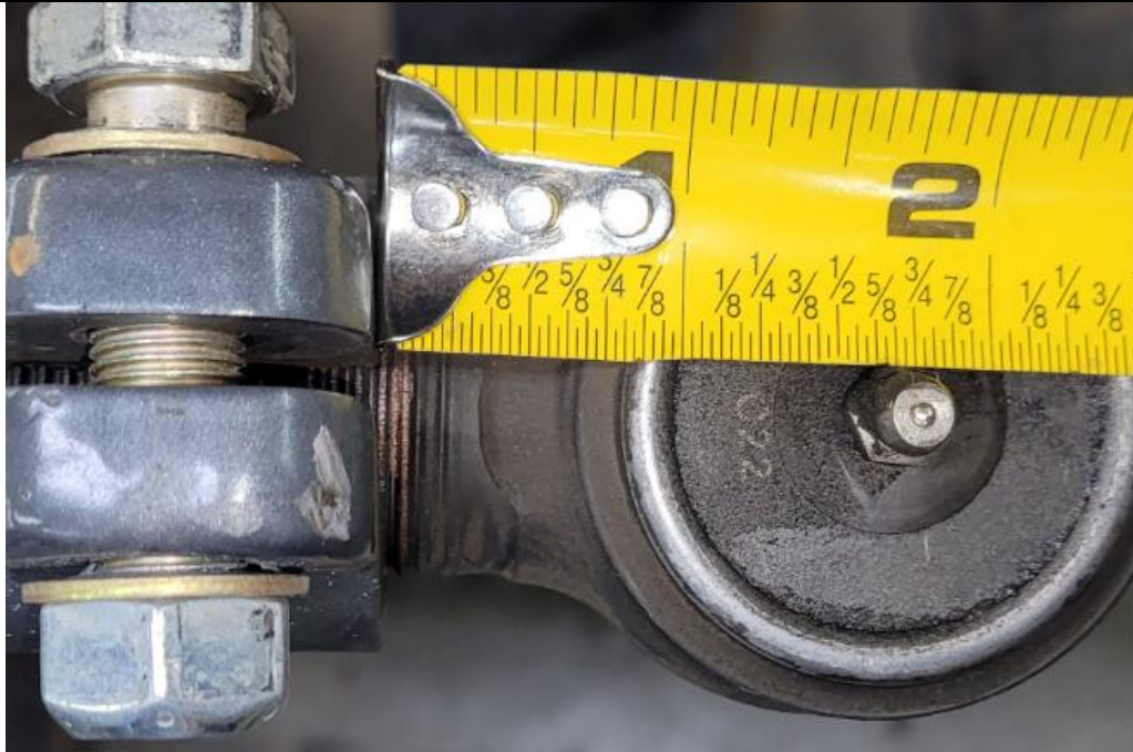
Figure 3. Driver's Side Tie Rod Minimum Length is 1-3/4" for 17" or 18" Rims.
