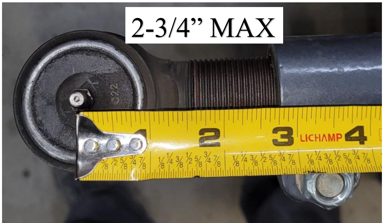
Figure 7. Driver's Side - NON-Double Adjuster Tie Rod End Maximum Extension
