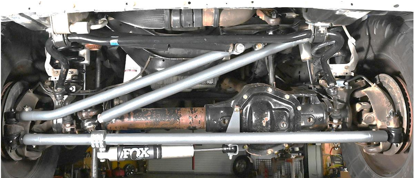
Figure 8. Completed Tie Rod Installation – Note: Synergy Drag Link, Track Bar, and Single Steering Stabilizer Mount are also shown
