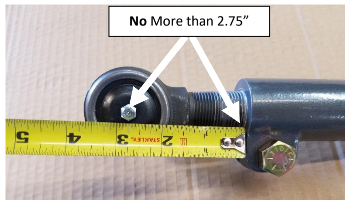
Figure 17. Tie Rod End Adjusted MAX 2.75" Out (Non Double Adjuster Side)
