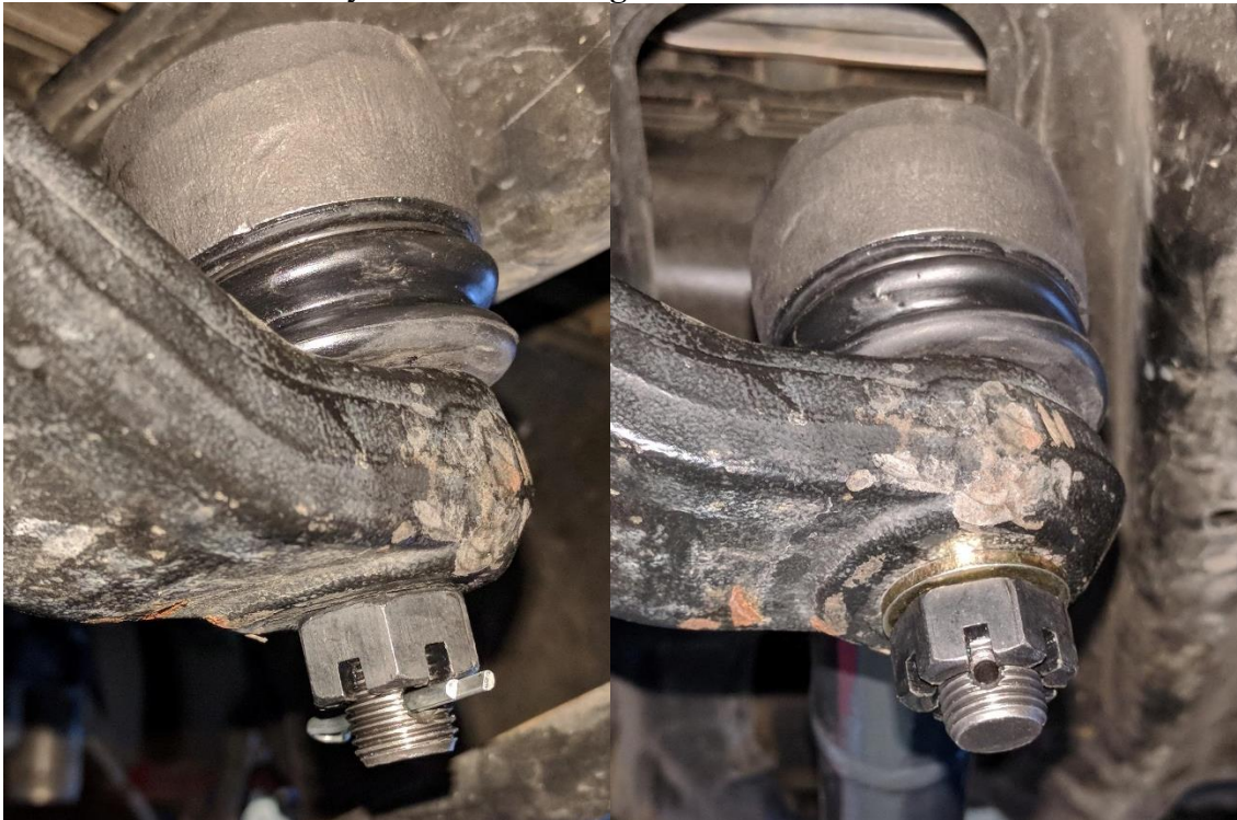
Figure 21 and 22. Washer Used Under Castle Nut
