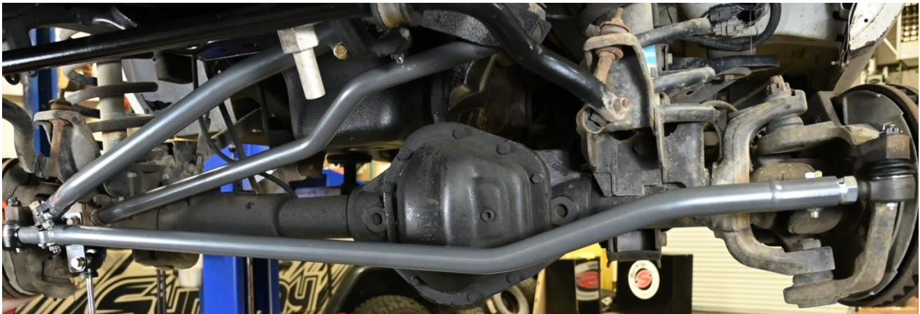
Figure 19. Installed Tie Rod and Drag Link
