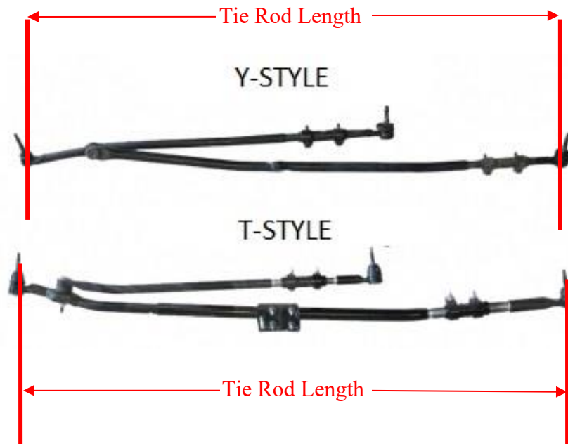
Figure 1. How to Measure Tie Rod Length
