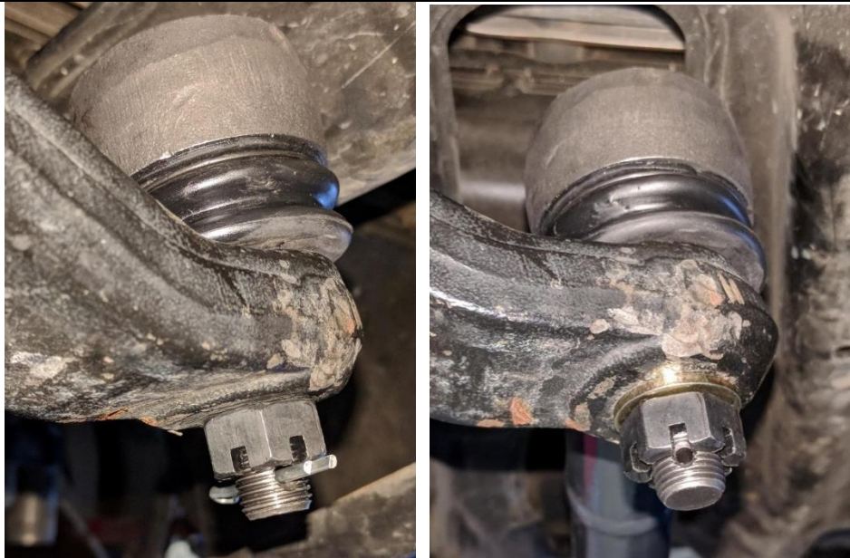
Figure 14 and 15. Washer Used Under Castle Nut
