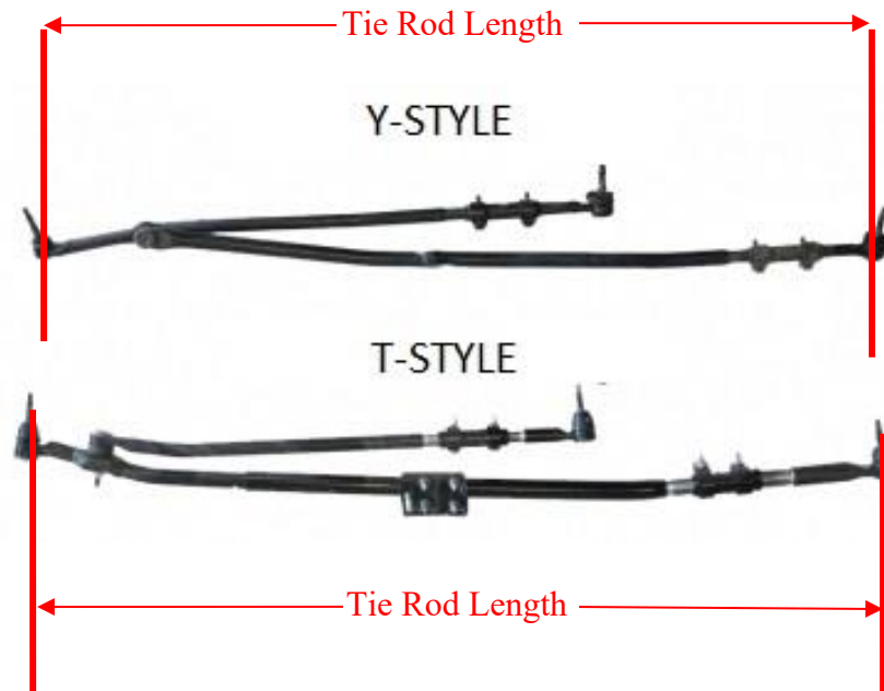
Figure 1. How to Measure Tie Rod Length
