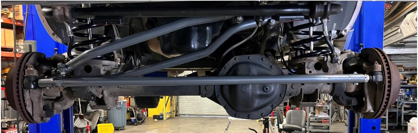
Figure 12. Installed Tie Rod and Drag Link
