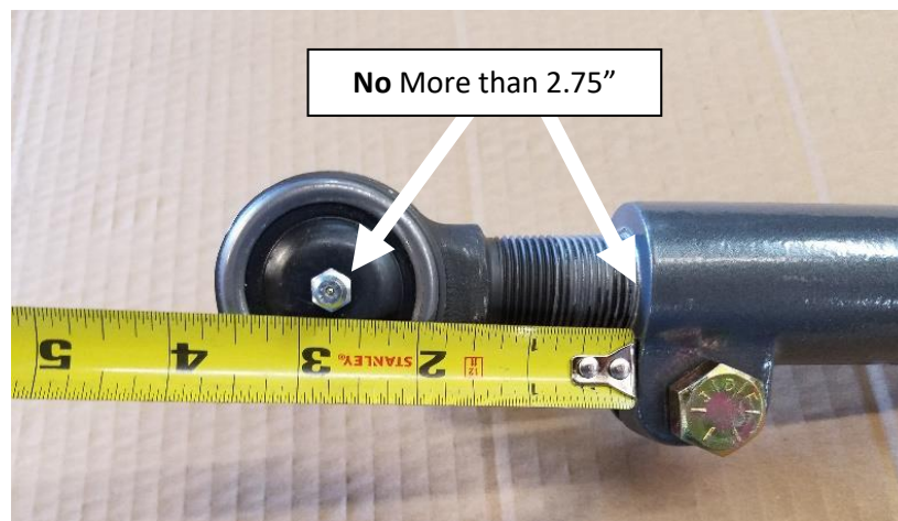
Figure 11. Tie Rod End Adjusted MAX 2.75" Out (Non Double Adjuster Side)
