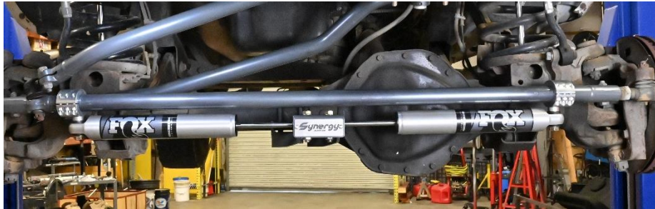
Figure 8. Driver Side Steering Stabilizer Installed on Dual Stabilizer Bracket
