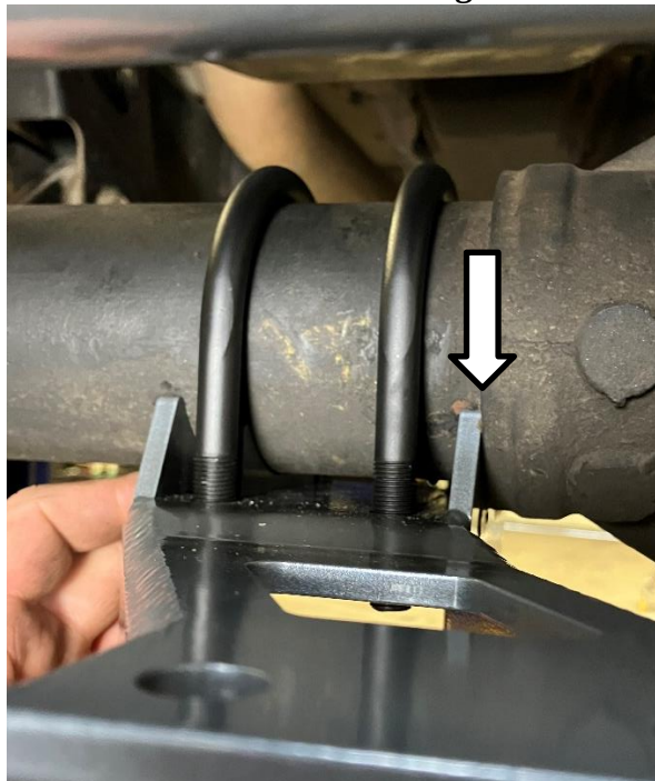
Figure 3. Dual Stabilizer Bracket Indexed on the Differential Housing
