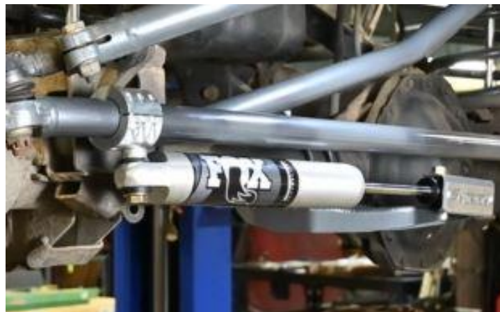
Figure 7. Correctly Installed Stabilizer
