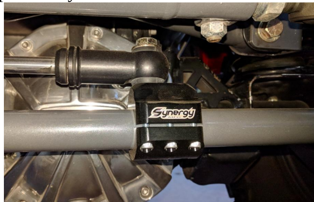
Figure 3. Synergy 8003-20 Clamp Installed On Tie Rod
