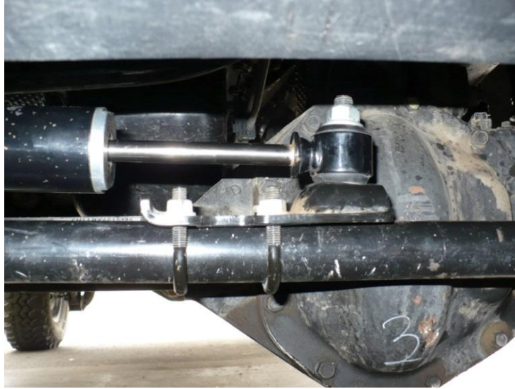
Figure 2. Factory Tie Rod Bracket ‘Flipped’
