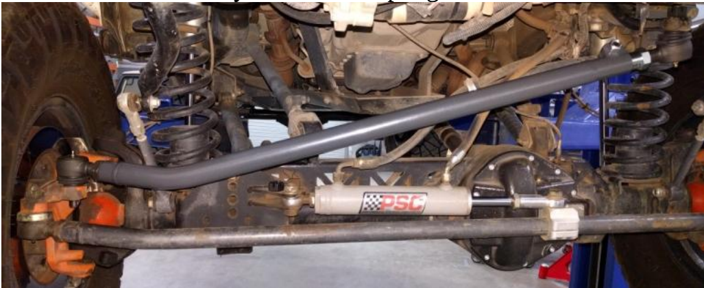
Figure 7. INCORRECT Orientation of Drag Link
