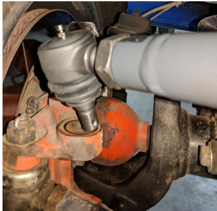
Figure 4. Drag Link at Knuckle End – Needing to be Adjusted to Fit
