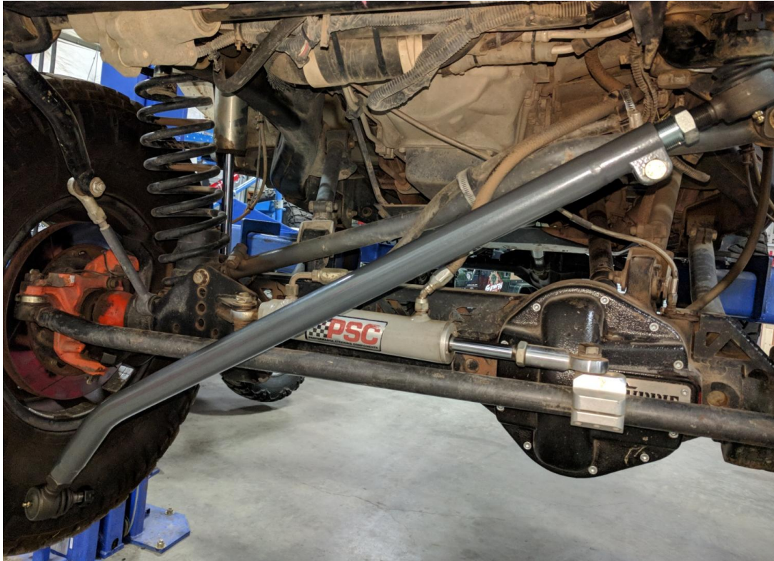
Figure 3. Drag Link Installed In Pitman Arm
