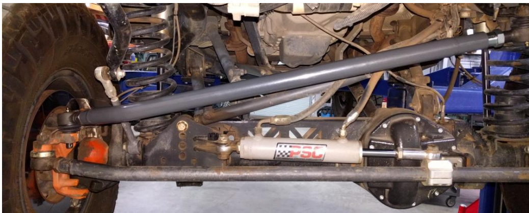
Figure 8. CORRECT Orientation of Drag Link
