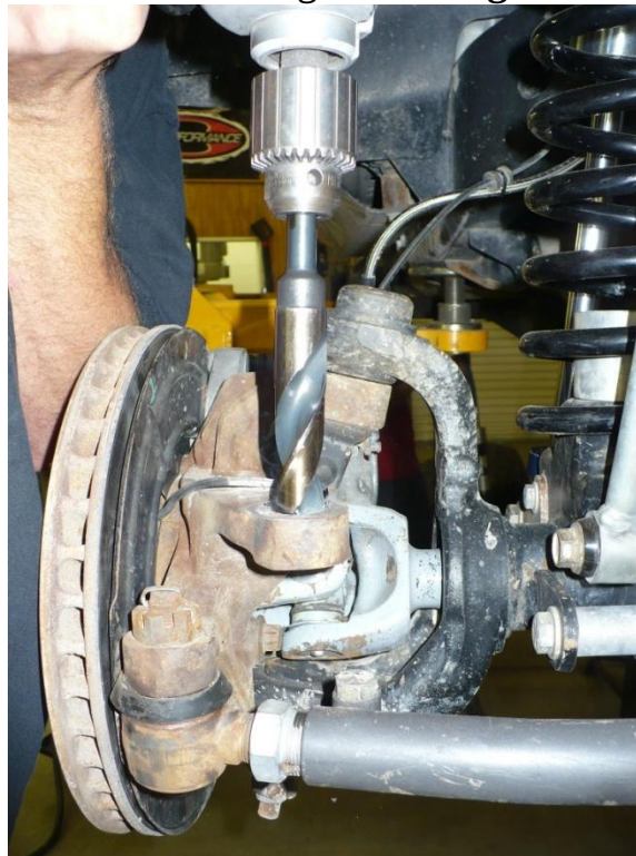
Figure 1. Drilling out Knuckle for Flip Adapter
