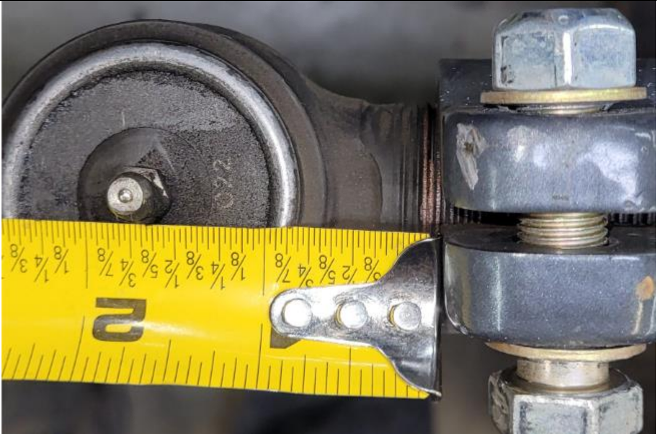
Figure 3. Passenger Tie Rod at Minimum Length for 17" or 18" Rims.
