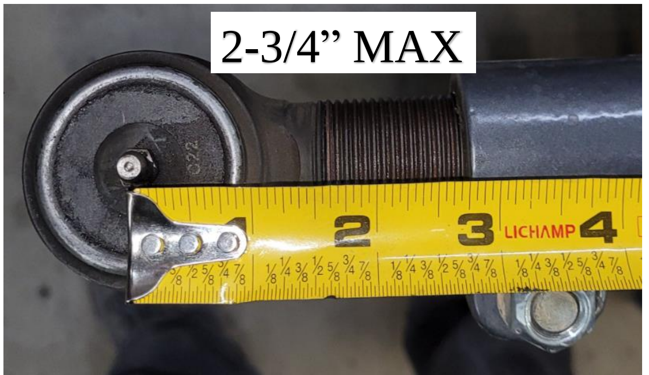
Figure 6. NON-Double Adjuster Tie Rod End Maximum Extension
