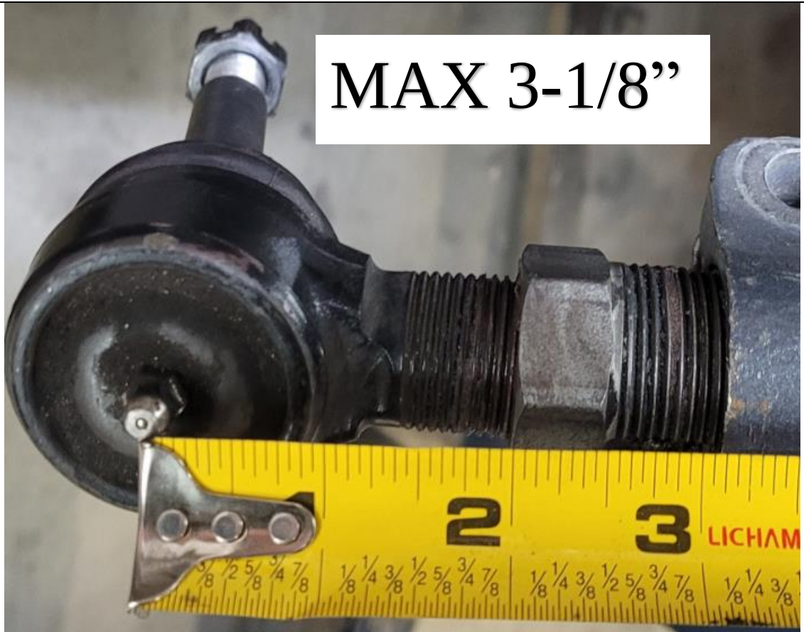
Figure 4. Double Adjuster Tie Rod End Adjusted to MAX 3-1/8\"
