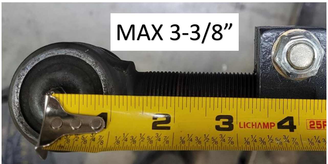
Figure 5. Non-Double Adjuster Tie Rod End Adjusted to MAX 3-3/8\"
