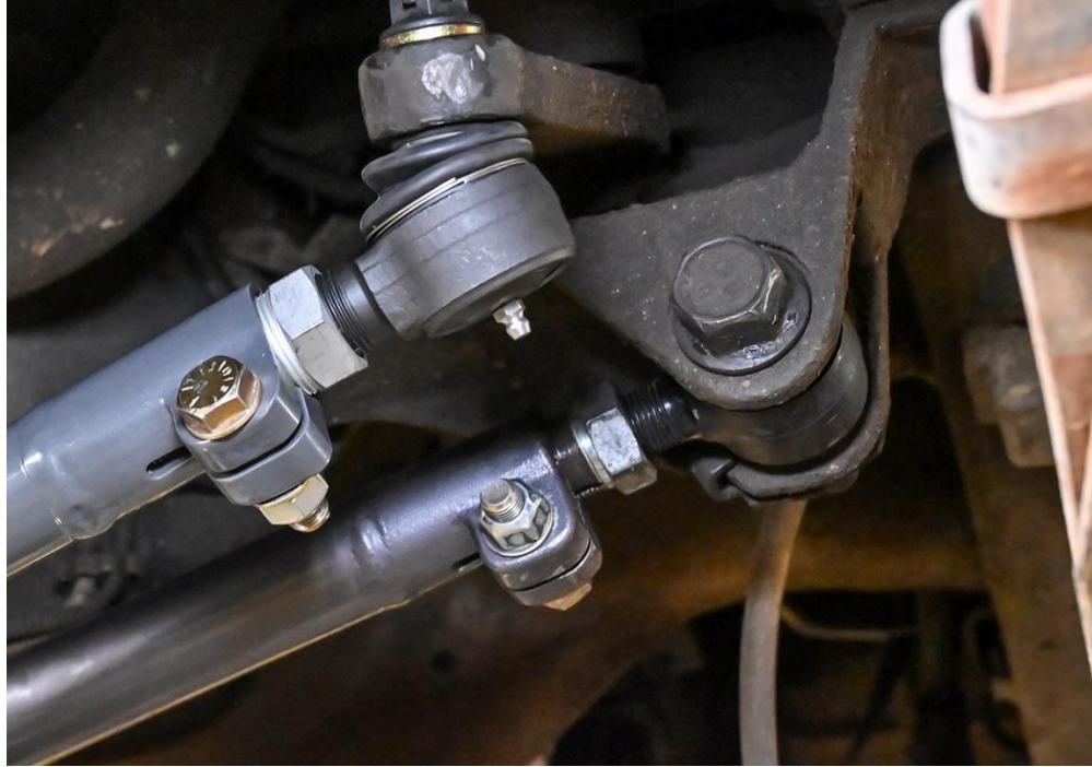
Figure 4. Installing the Frame Side Bolt and Nut
