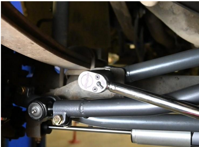
Figure 5. Torquing Axle Side Bolt
