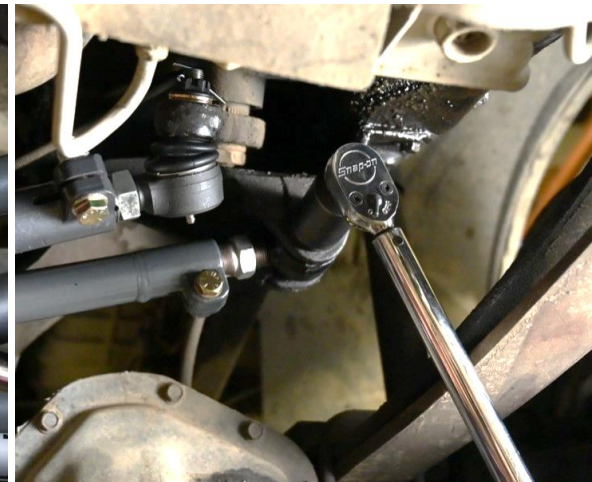
Figure 6. Torquing Frame Side Bolt
