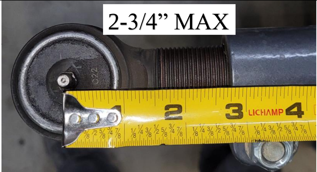
Figure 3. NON-Double Adjuster Tie Rod End Maximum Extension
