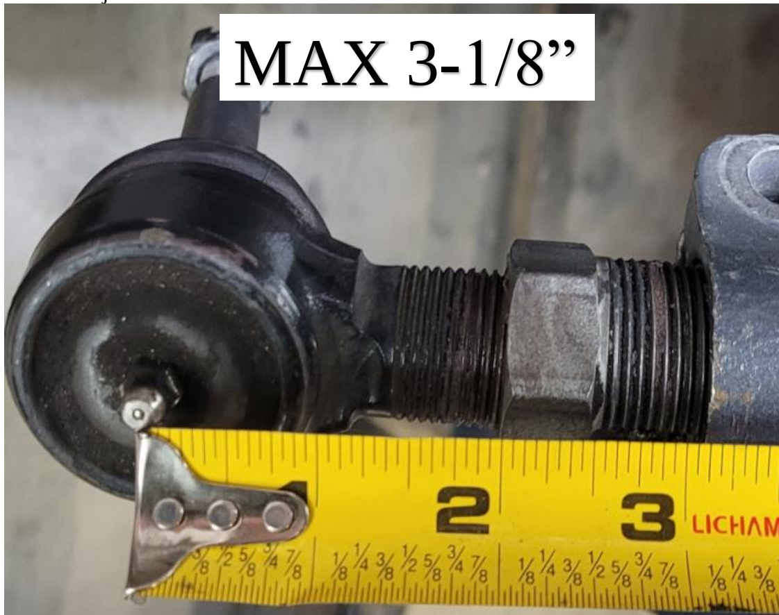
Figure 2. Double Adjuster Tie Rod End Maximum Extension.
